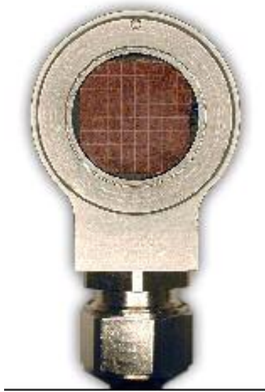
Figure 3.1 A picture of the matrix transducer used in the non-destructive spot weld detector application.
