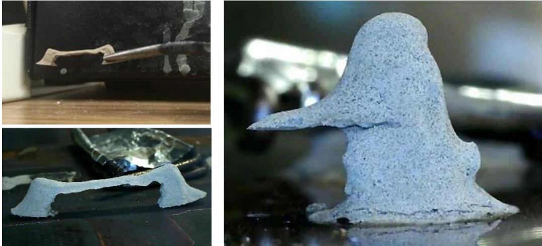
Figure 3-4: Self-supporting 3d bridges and cantilever beams were printed with a series of 3-4 min heating cycles at 130°C followed by 2 hr. sintering at 300 °C using a support structure of Al foil on Cu wire.
