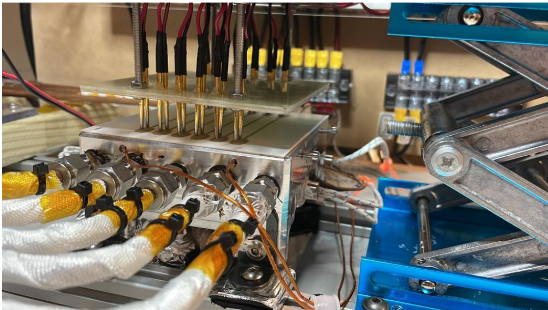
Figure 4-15: The figure shows the compressed-state of the current probe configuration. The compressed state supplies cumulative downward force against the alumina board that improves the heat transfer from the hot-plate.
