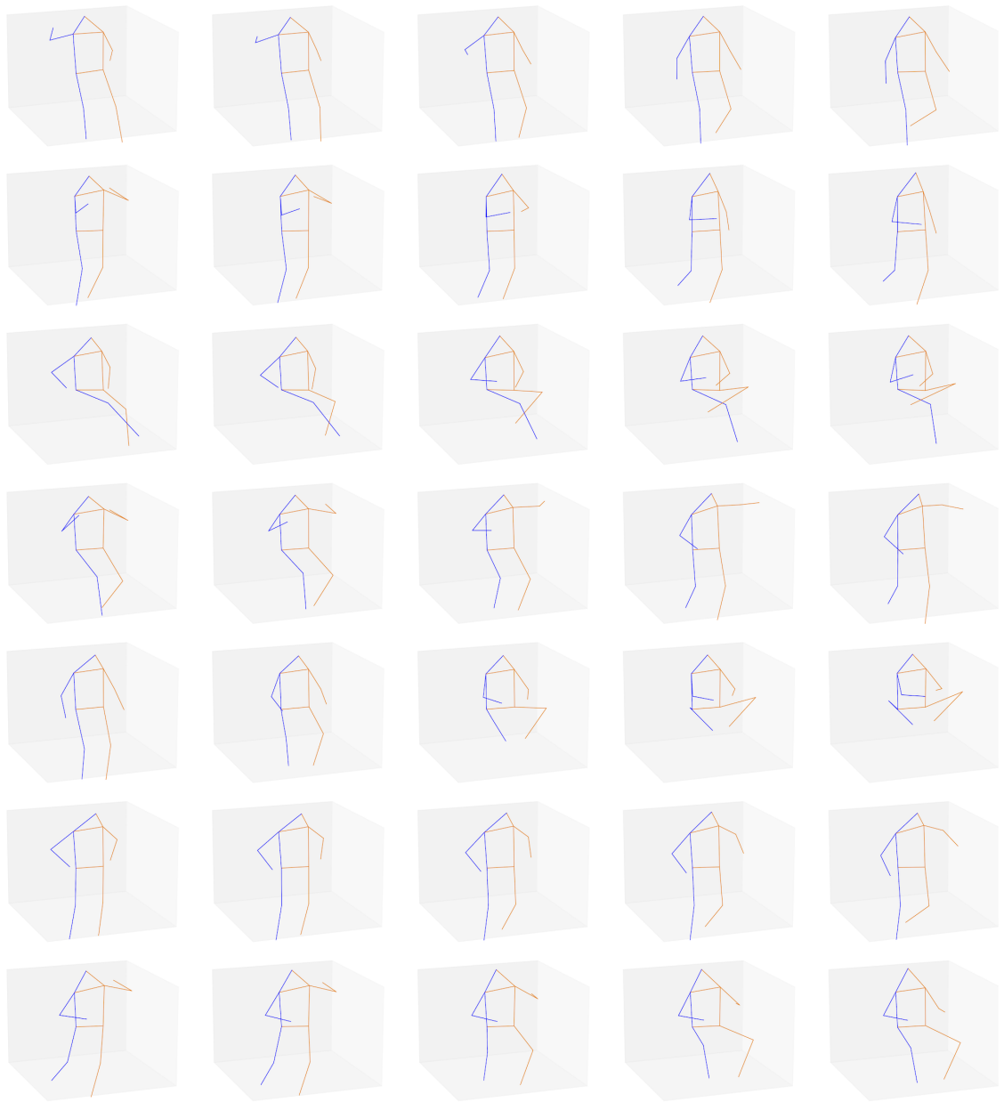
Figure 2.10: Given the frame on the left and the frame on the right for each example we show our models ability to generate frames in between two poses. We take the mean for the embedding space of two poses, calculate the distance between those two means and then add a portion of the distance to the embedding on the left at each step. The images seen in the middle three columns are all generated. We can see that we are able to generate a sequence of poses that lead from one random pose to another.
