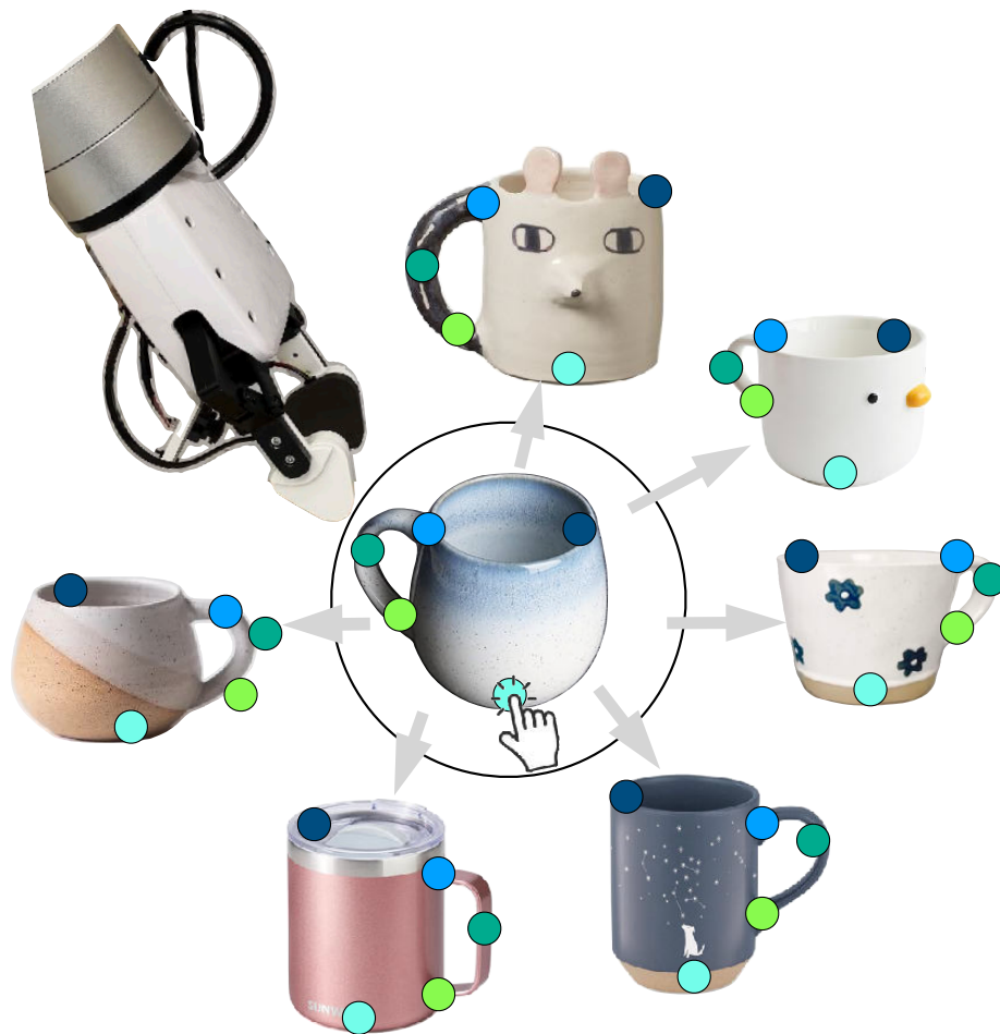
Figure 3.1: A human prescribes key points one time for one instance of an object and those points are transferable to all other instances of the same object.
