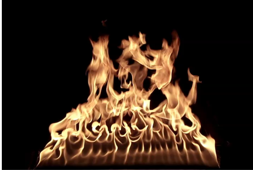
Figure 1.1: Streaks in flame show both vortex and wave instabilities in experiments using an inclined porous gas burner of width 0.595 m [1].
