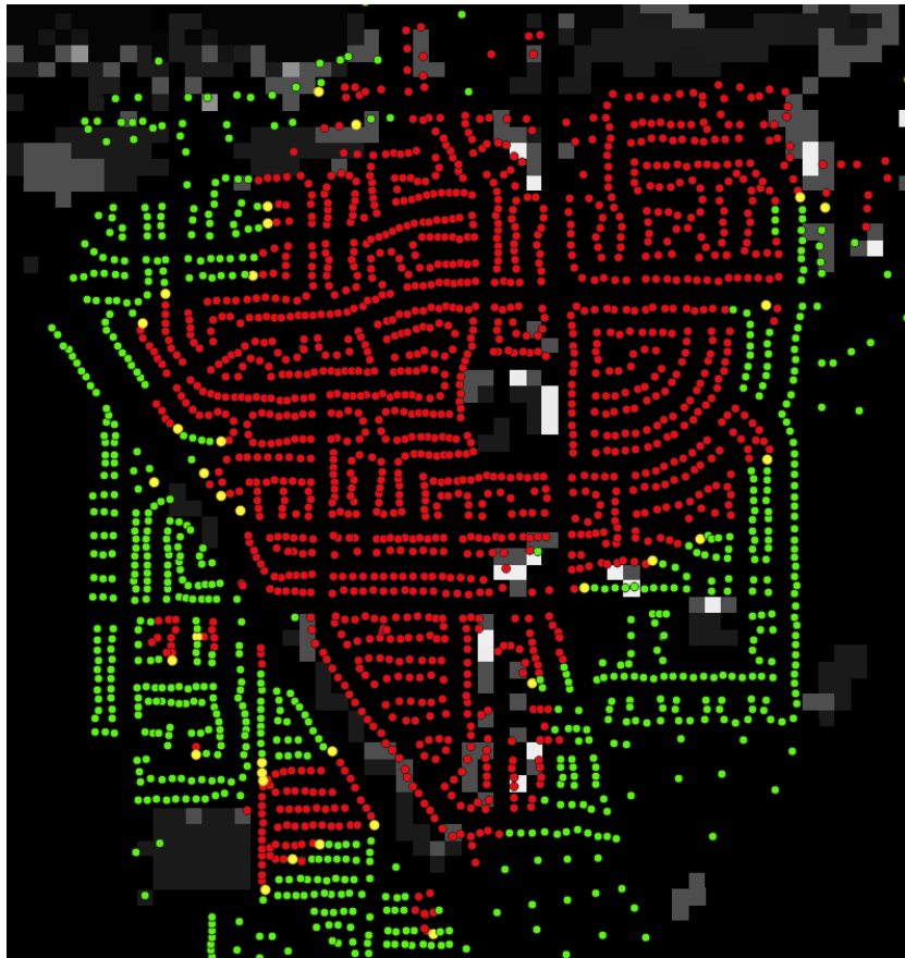
Figure 6.20: Coffey Park, structures color-coded by damage state (green = undamaged; yellow = partially damaged; red = destroyed) overlaid on the area fuel models, where black represents non-burnable fuels and lighter grays and white represent a variety of burnable fuel models. Most of Coffey Park is shown to be non-burnable, including areas with destroyed structures.
