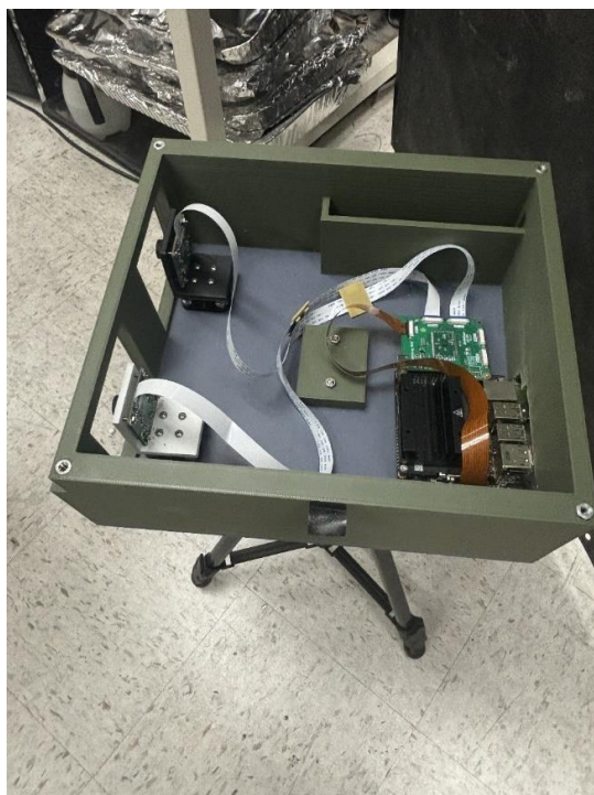
Figure 23. Alternative view of the ember flux meter.
