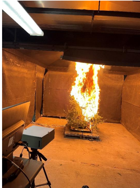
Figure 8. A Christmas tree burn test being filmed by the stereo vision cameras.
