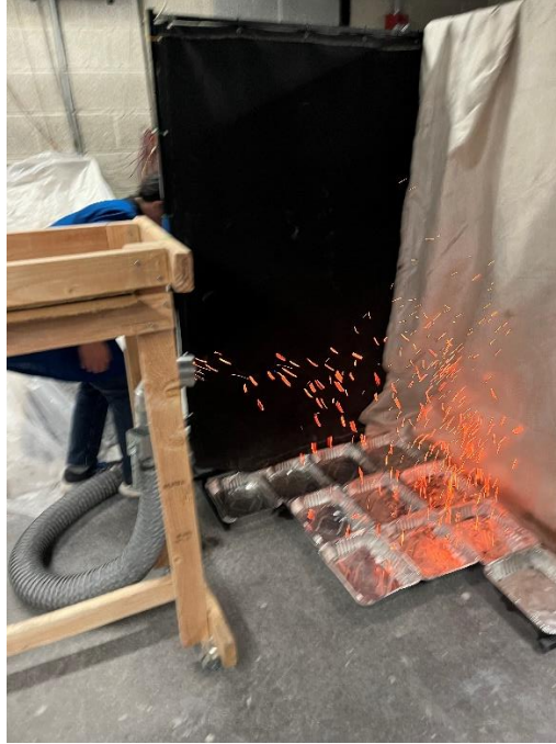
Figure 6. An ember shower produced by the second iteration testing setup.
