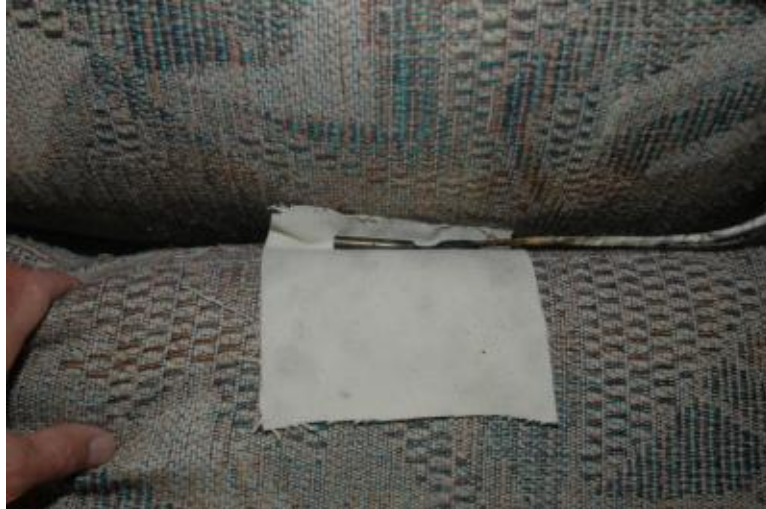
Figure 5-20. Cartridge heater setup for test SM4
