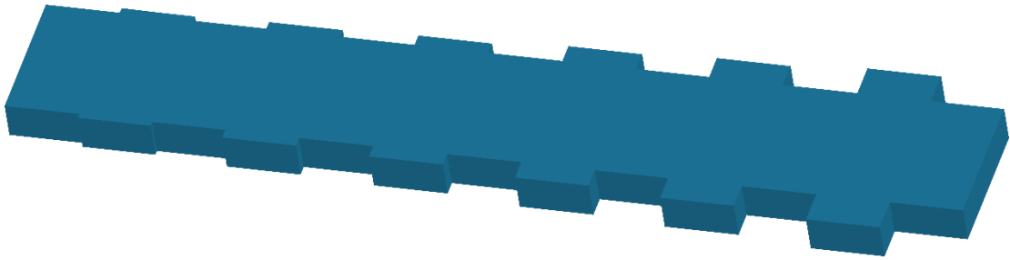
Figure 8.12 Schematic illustration of a taper Bragg grating.
