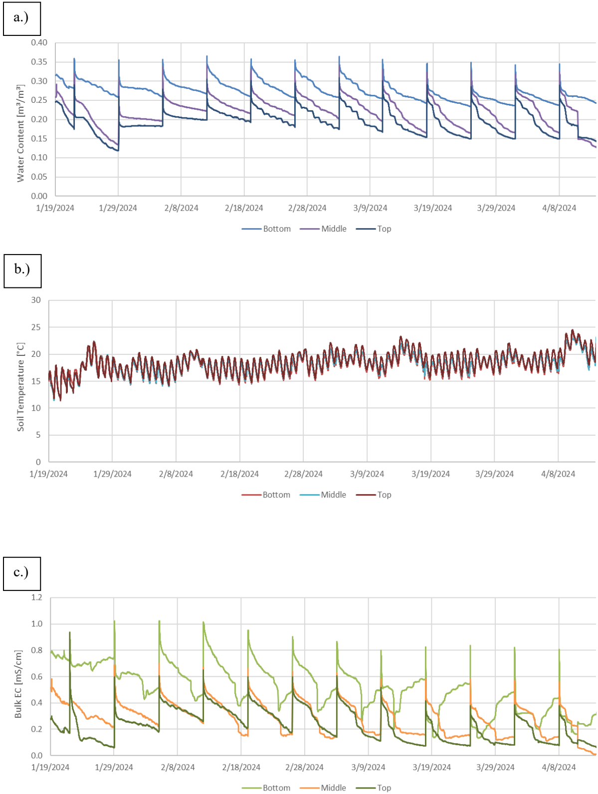
Figure E.3: Soil sensor readings for SL. a.) water content, b.) soil temperature, and c.) soil bulk electrical conductivity (EC).
