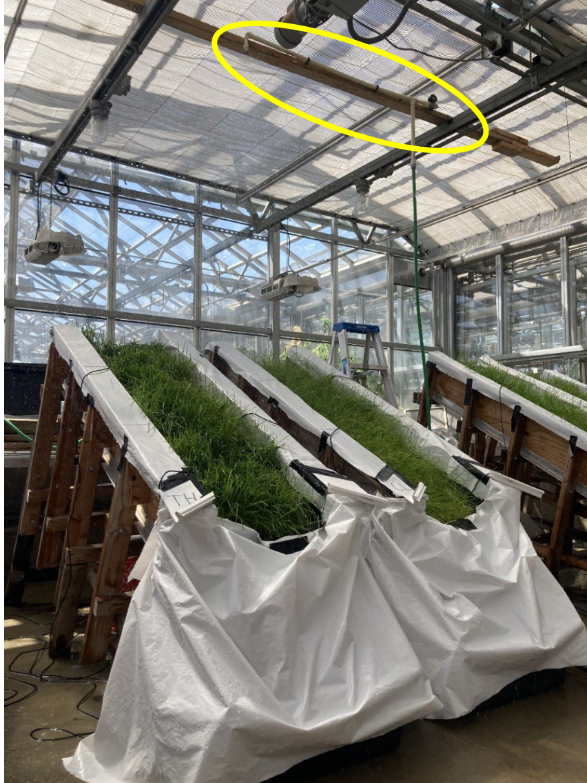
Figure 2.9: Mesocosms TH and CL with rainfall simulator (circled) during rainfall event 12.
