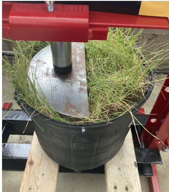
Figure 2.5: Hydraulic press and semi-circular plate applying compaction load to pot.
