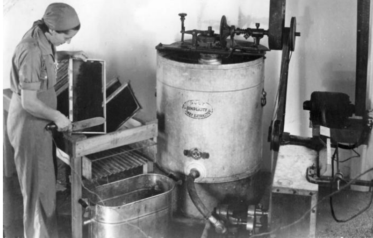
Figure 3.9 The process of uncapping wax with a knife and honey being extracted using a multi-frame electronic extractor. (Source: Joshua Hennig, 1954)
