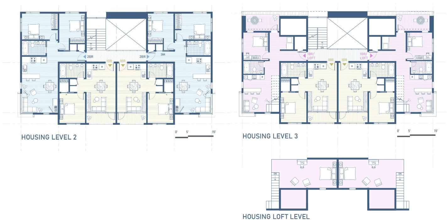
Figure 49: Live/work housing floor plans illustrating the spatial organization, residential typologies, and mixed-use framework supporting Gloucester's fishing community. Drawings by author.
