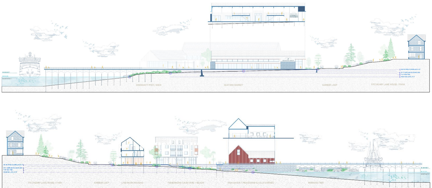
Figure 44: Site sections illustrating the relationship between topography, floodplain conditions, public waterfront space, elevated habitable programs, and resilient coastal edge strategies within the proposal. Drawings by author.
