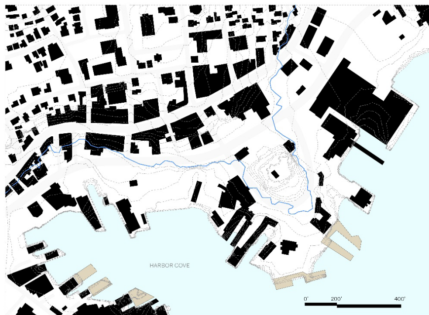
Figure 34: Existing figure-ground and topographic analysis of the selected waterfront site in Gloucester illustrating the FEMA 100-year floodplain elevation (14 ft), existing urban fabric, waterfront infrastructure, and vulnerable low-lying coastal edge conditions surrounding Harbor Cove. Diagram by author.
