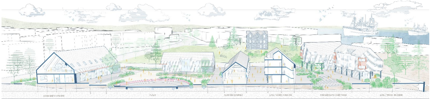
Figure 43: Longitudinal site section perspective illustrating the spatial relationships between community programs, public open space, seafood market, fishermen's housing, and the working waterfront within the proposed harbor framework. Drawing by author.
