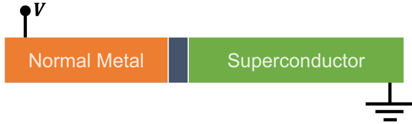
Figure 1.4: Schematic plot of the normal metal-superconductor (NS) junction. A bias voltage is applied to the normal metal, with the superconductor grounded.
