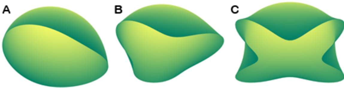
Figure 3.1: (A) The first buckled mode shape of the hemisphere, which is the only naturally apparent buckling mode without boundary stimulus. (B) the second (3-lobed) buckled mode shape of the hemisphere. (C) the third (four-lobed) buckled mode shape of the hemisphere.
