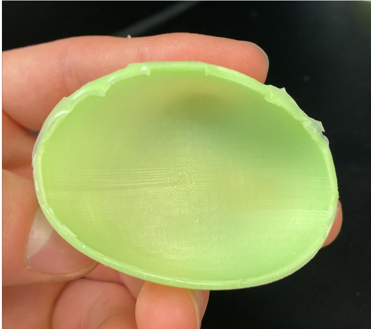
Figure 2.4: A hemispherical shell manufactured using a mold-and-cast technique
