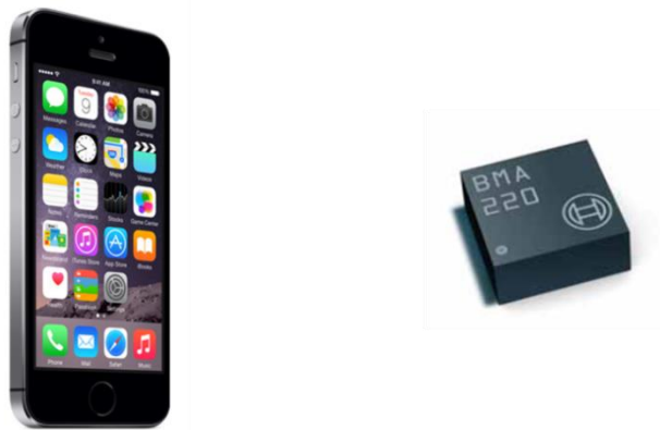
Figure 5.3: iPhone 5S Accelerometer – BMA220 (Bosch Sensortec, 2011)
