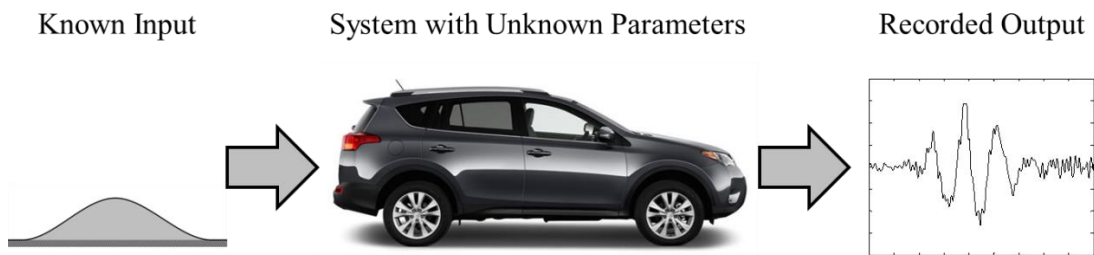
Figure 5.1: Testing Process for Known Input
