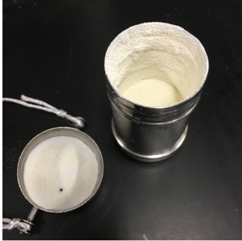
Figure 4.4: The canister in which grains are charged in our experiment. The interior of the canister has been coated with grains of the same material as those to be charged, so that no grain-to-wall charging occurs. When the lid is rotated during sample collection, grains fall through the 5 mm hole in the lid at bottom left.
