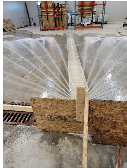
Figure 4-1. Viking Bucket Test Setup
