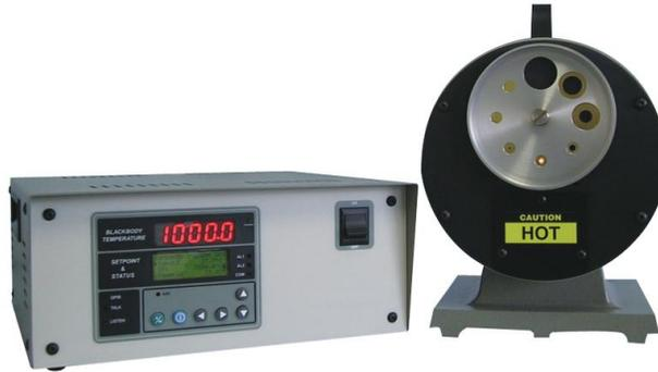
**Figure 2-2: Commercial blackbody furnace used in the experiment**
