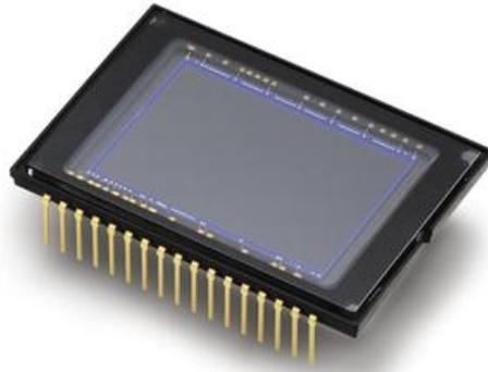
**Figure 1-3: CCD sensor used in Nikon D100**
