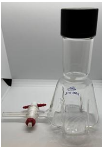
Figure 2.4. Photograph of a 250 mL baffled flask that is used in the Baffled Flask Test (BFT) for determining the efficiency of oil-dispersion.
