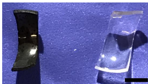
Figure 2.S13 Optical images of macroporous pristine PNIPAM hydrogel sheet (right image) and hybrid hydrogel sheet (left image). It can be seen that the gel surface of the hybrid sheet is dark and shining (rather than transparent as the pristine hydrogel sheet without Ag nanoparticles), indicating the presence of a high-density AgNPs on the sheet's surface. Scale bar: 0.2cm.
