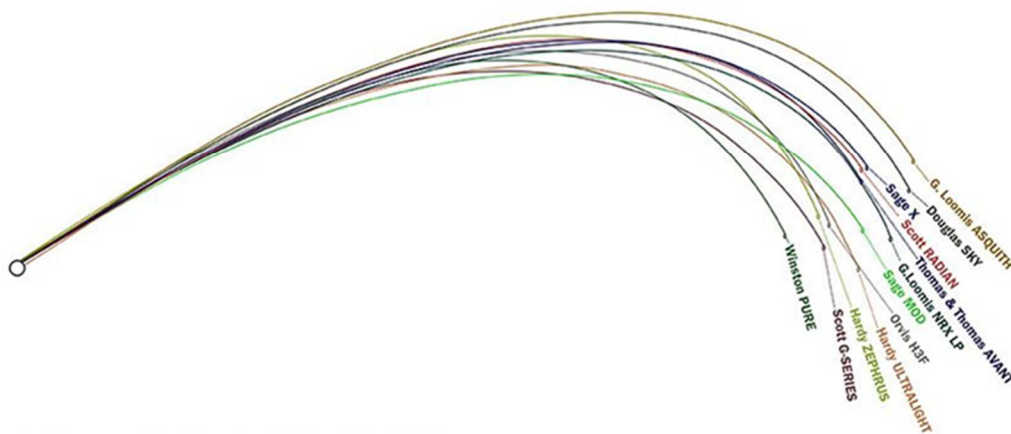
Figure 6 – Fly rod deflection curves [6]
