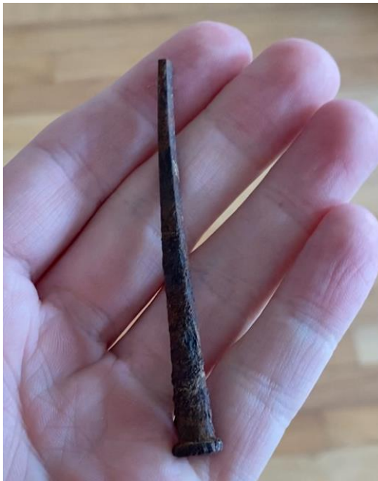
Figure 29. Mid-nineteenth-century cut nail removed from rafter in Phase II attic (Grant Cunningham, 2022).
