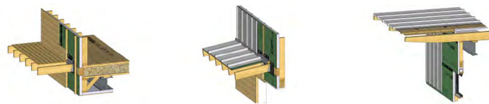
Studies of hybrid steel + wood structural components (Davies and Knoebel)
