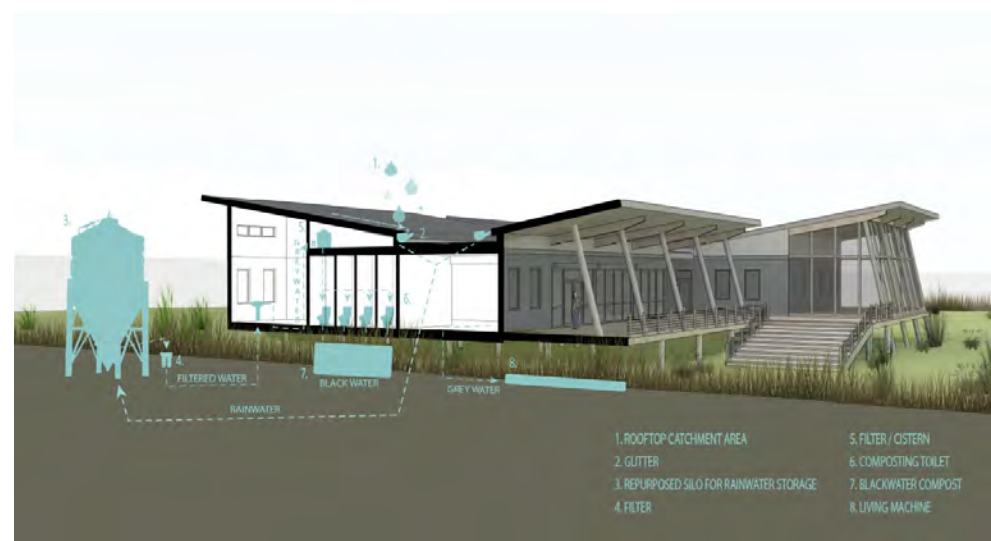
The roof form captures rainwater and stores it in the re-purposed silos. It is then filtered and treated using UV light and distributed back into the labs, bathroom and kitchen sinks, showers and toilets. The greywater from sinks and showers is piped into a living machine on the southwest side of the building that uses native plants to filter the water. (Robbs and Peters)
