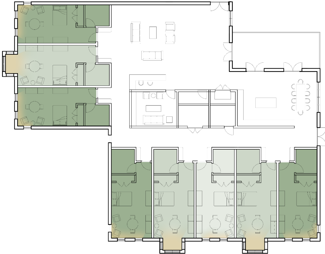
Figure 49: Community A Daylighting (Source Author)
