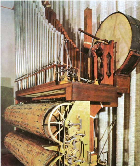
Figure 35: The Componium, showing the composition barrels
