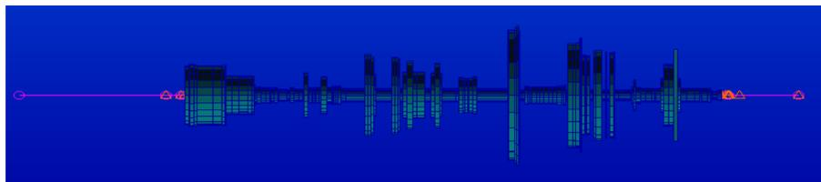
Figure 3.10: NASTRAN FE model of GE CT7-8 engine
