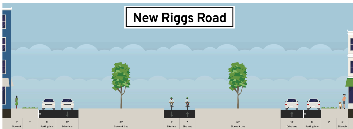
Fig 81. Proposed dimensions for the street layout of the northern section of New Riggs Road. Created using Streetmix, 2024.
