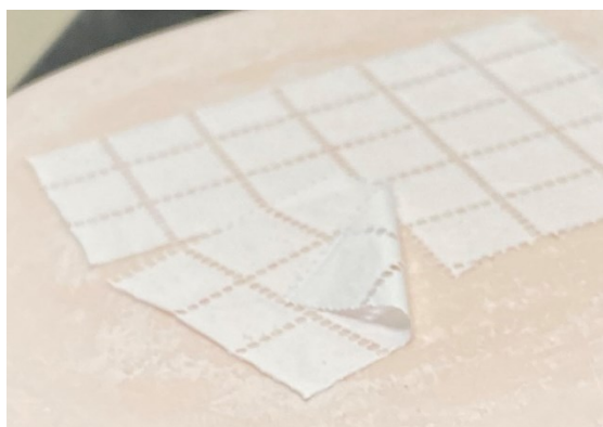
Figure 37. Post sintered separator structure displaying flexibility.
