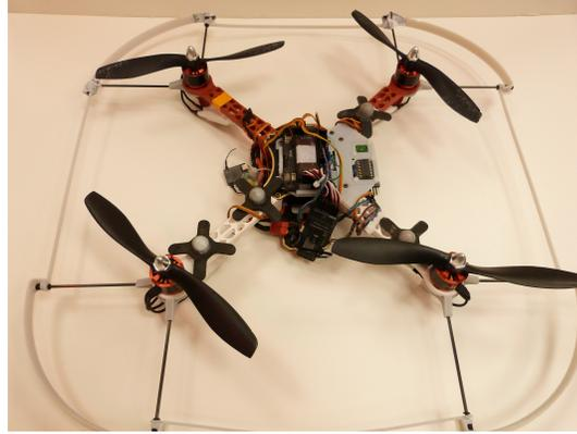
Figure 6.2: FlameWheel 330 commercial quadrotor with Ardupilot attitude control board.
