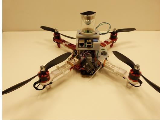
Figure 6.4: Flying vehicle hardware integration.
