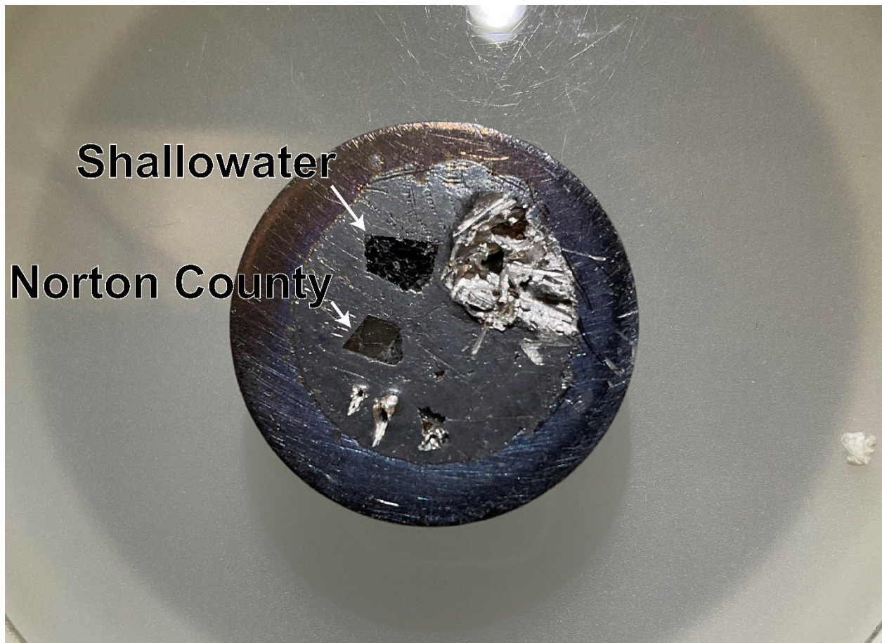
Fig. A11) Reflected light image of 1 inch indium mount holding Norton County and Shallowater. The three small holes held the secondary standards Suprasil 3002, Herasil, and ALV-519-4-1 glass. The large hole held a sample that was not used in this study.
