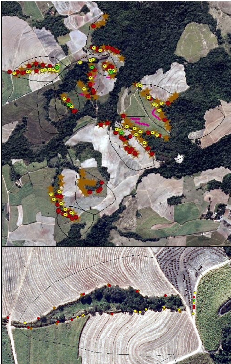
Figure 1.8 (a) Berms extremities (stars) and erosional features (dots: permanent gullies-red, ephemeral gullies-yellow, and rills-green) within study catchments. Pink lines are continuous erosional features within sugarcane fields (top). (b) Detail of one of the study catchments (P7) to show that gullies were occurring at berms extremities (bottom)
