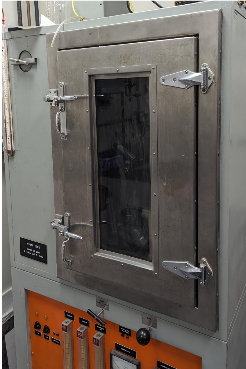
Figure 6.3 ASTM E662 chamber used for UMD tests
