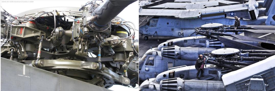
Figure 1.2: CH-53 Rotor Swashplate
