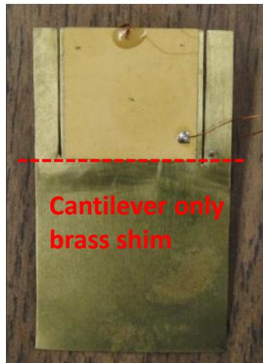
Figure 2.35: PZT-5K4 Bimorph with No Piezoceramic in Cantilever ('Dead')
