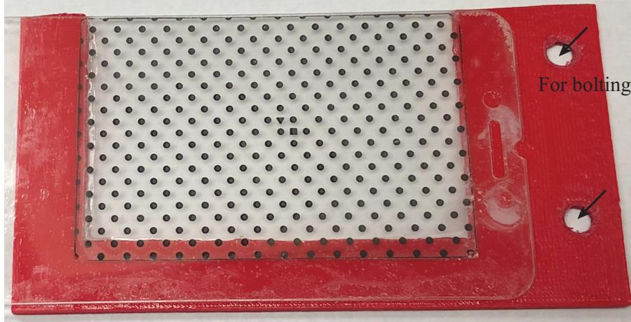
Figure 4.6: Photo of the printed calibration target on a transparent polymer film sandwiched between two glass slides.
