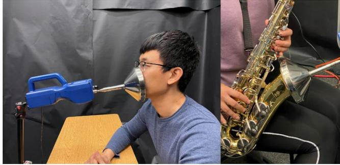
Figure 5 Source aerosol measurements with funnels for singing (left) and instrument (right)
