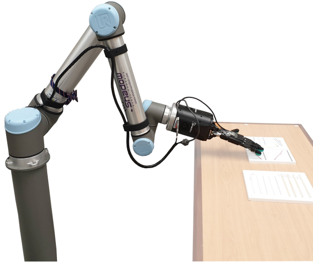
Figure 4.3: Hardware Setup: Shadow Hand mounted on UR-10 manipulator ground-truth timestamps for slip events.
