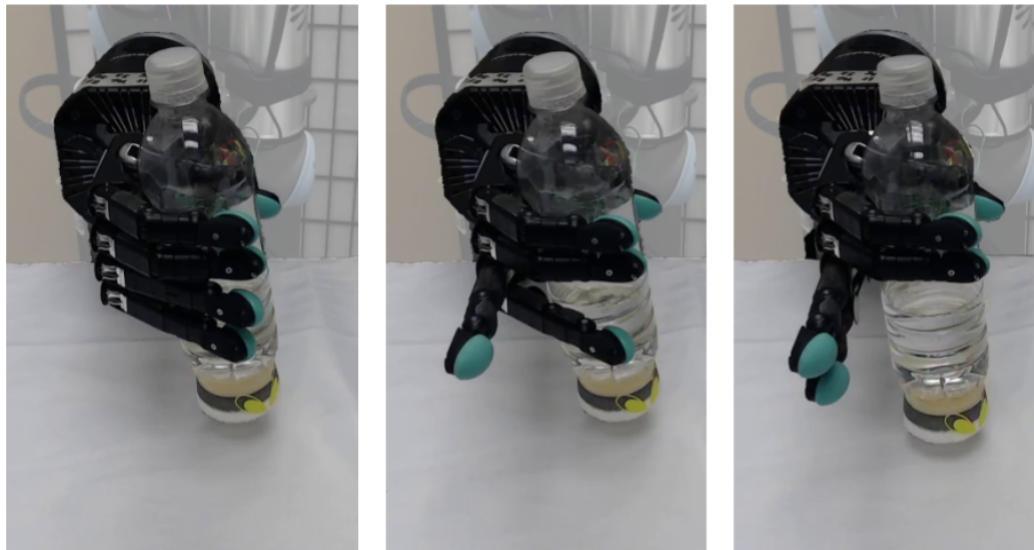
(b) Demonstration of the stable grasp as the number of fingers contacting the object are reduced.
