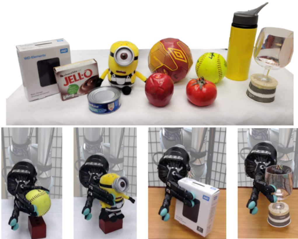
(a) Top: Dataset of objects used in experiments. Bottom (L-R): Grasping of Softball, Soft Toy, Box and Wine Glass.
