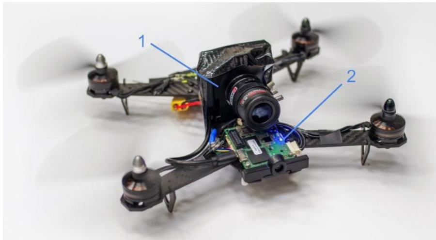
Figure 3.7: *Drone used in the dataset collection. 1 - mounted DAVIS240B camera, 2 - Customized Qualcomm Flight platform with onboard computer*
