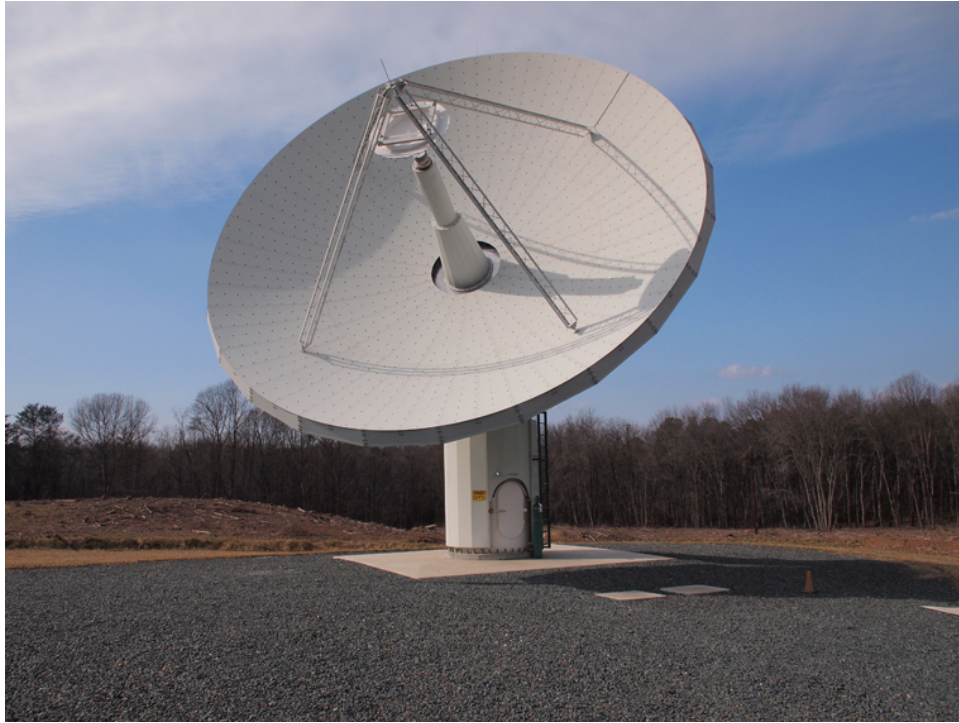
Figure 3.1: Photo of the 12 m GGAO VGOS antenna (courtesy of NASA SGP)
