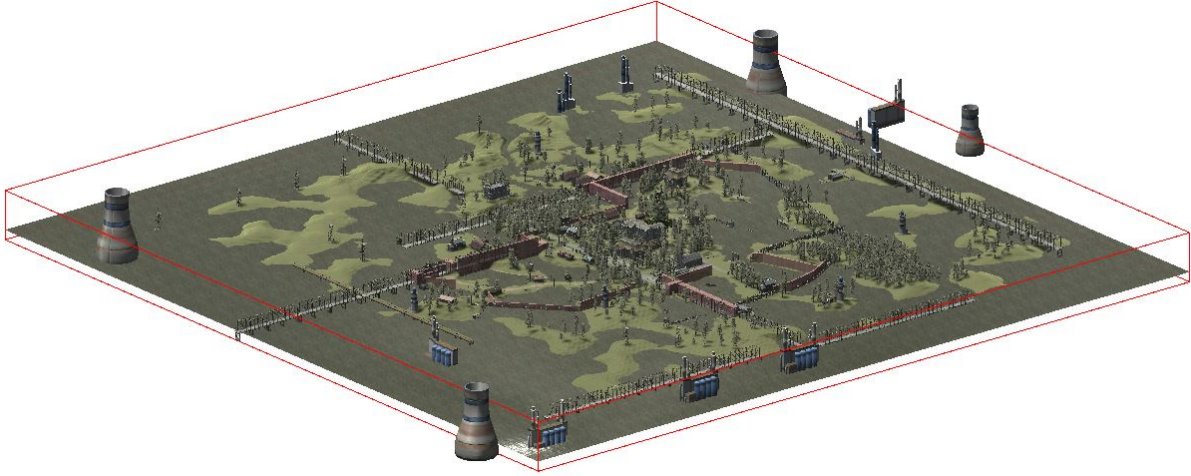
Figure 6.3: Overview of the chosen boundaries (red) for the 3D raster search applied to the complex scene to include the entire environment.
