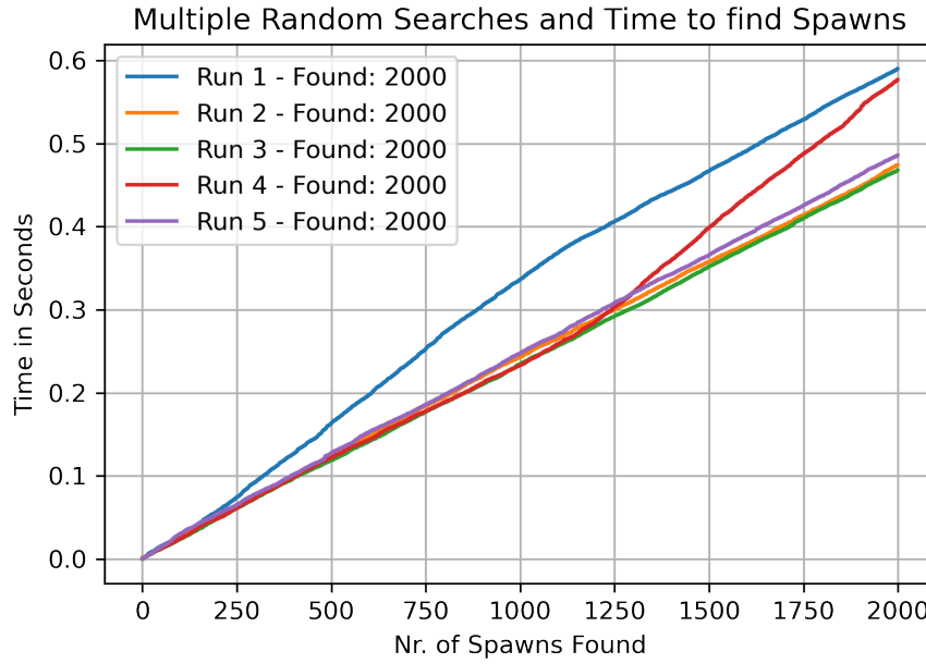
Figure 6.11: Test of the random search algorithm without distance check for previously checked locations.
