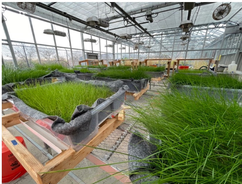
Figure 4.2. Simulated rain events equivalent to 25.4 mm of rainwater were applied biweekly to greenhouse microcosms to measure nitrogen and phosphorus leachate totals from fertilized soil or soil amended with one of four biosolids treatments: new biosolids, new biosolids and wood fines, or old biosolids and wood fines. Microcosms were designed to collect leachate in plastic gutters that diverted it to 22.7 L plastic collection buckets.
