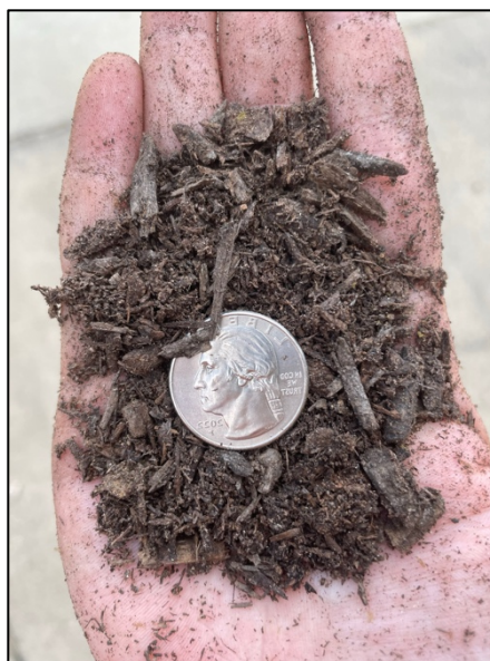
Figure 5.1. Recycled wood fines (WF) were blended 1:1 with old biosolids to form the OBWF amendment. Likewise, they were blended with fresh biosolids to form the NBWF amendment
