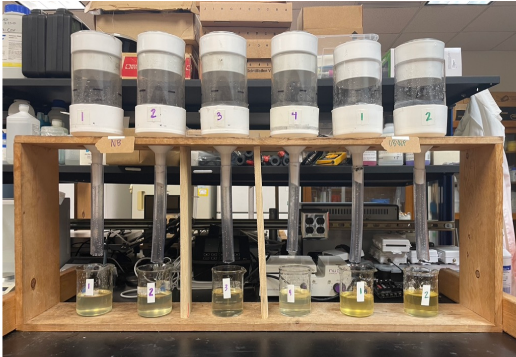
Figure 4.1. A column study was conducted to determine nitrogen and phosphorus losses from four soil amendments: new biosolids, old biosolids, new biosolids with wood fines, and old biosolids with wood fines. Columns were loaded with soil to a depth of 63.5 mm and received a total of 1.75 L of deionized water, the equivalent of 158.8 mm of simulated rainfall, over 5 weekly leaching events.
