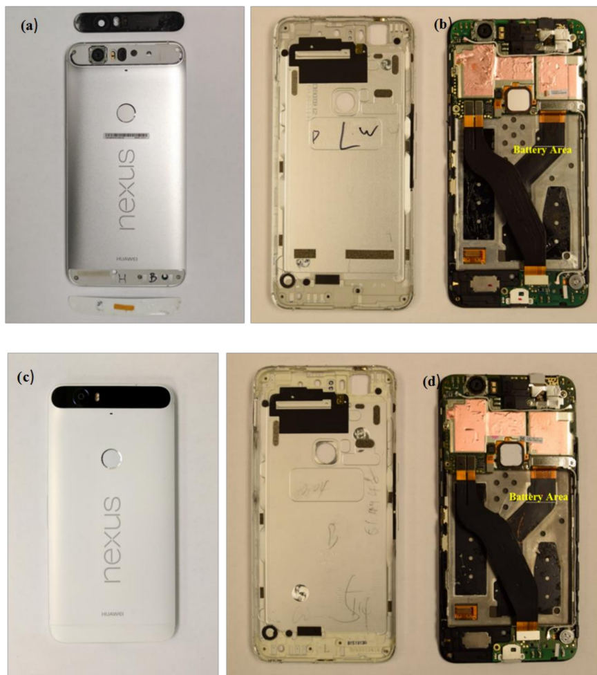
Figure 1. (a) Back cover of the new smartphone; (b) separated back and front panels of the new smartphone; (c) back cover of the used smartphone; (d) separated back and front panels of used smartphone.
