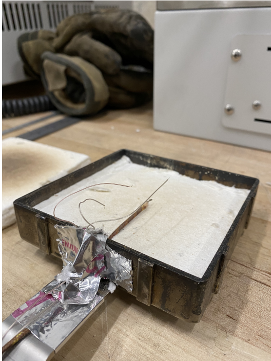
(a) 40 Gauge and 24 Gauge Thermocouples
