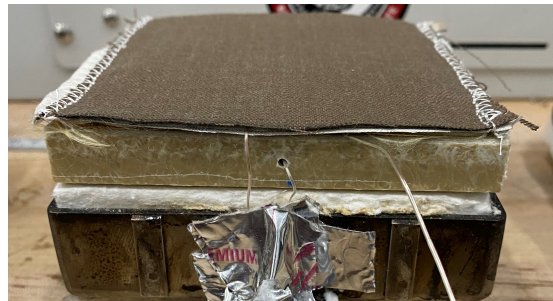
(c) Inserted Thermocouple Wiring
