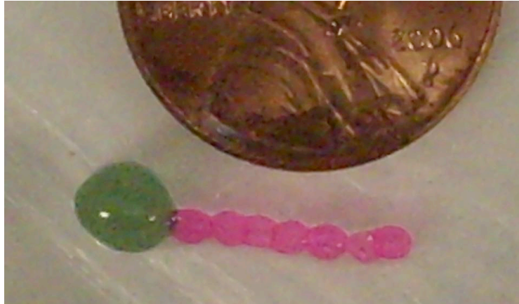
FIGURE 1.1. A biomimetic “earthworm”-like structure composed of linked capsules. The structure features a big green magnetic head linked to a chain of pink non-magnetic spheres. The big magnetic head allows for easy maneuverability by an external magnetic field in a liquid medium.
