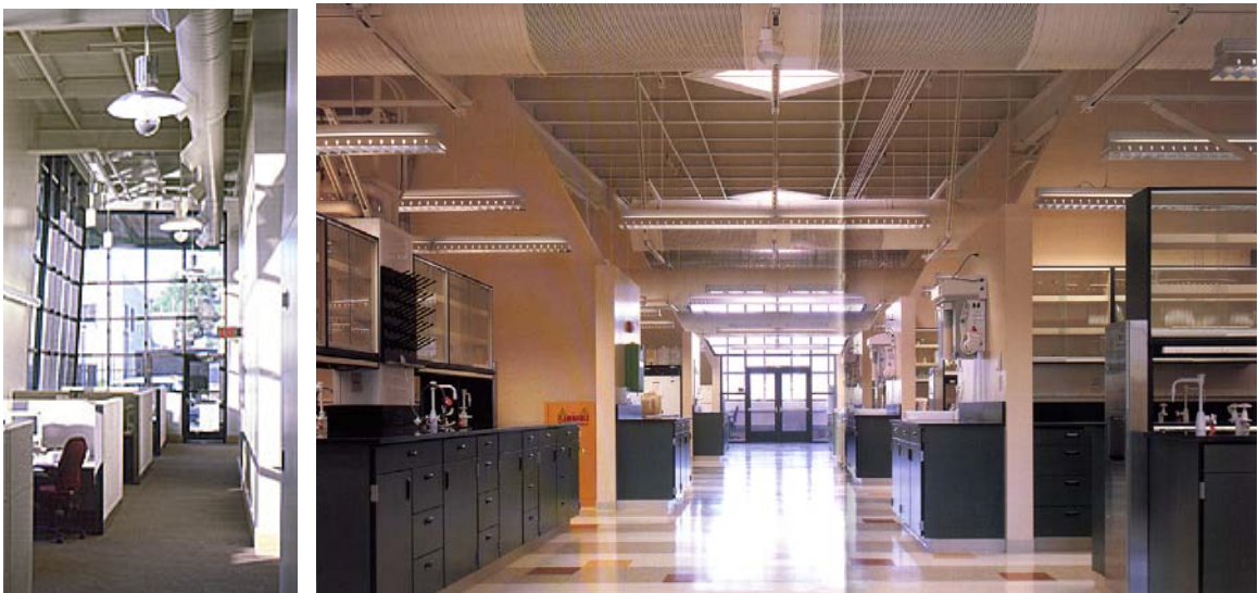
Figure 48 View of open plan office space 13 (left) and Laboratory 14 (right). Office is placed where natural light can be used. In addition to the skylights, glazed doorway separating public corridor and laboratory space brings natural lighting into laboratory area.
