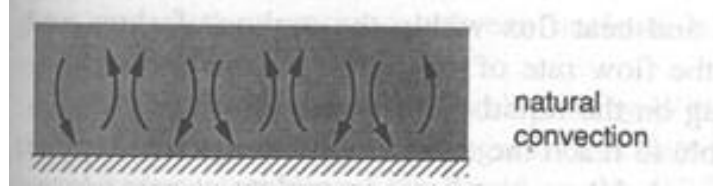
Figure 1.3: Schematic of natural convection and the onset of boiling (Carey, 1992).
