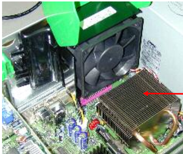
Figure 1.1: Thermosyphon in computers (Coursey, 2003).
