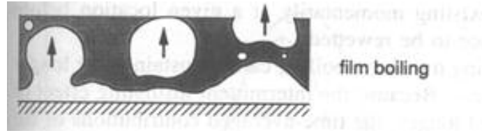
Figure 1.9: Schematic of film boiling (Carey, 1992).
