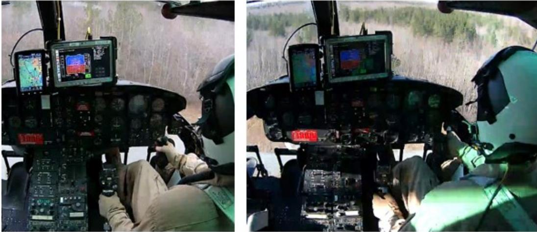
Figure 4.12: Two Images from the System Under Test Taken at Roughly the Same Point During the Scripted Demonstration. The Left Image was Taken on 12 December 2017 and Depicts the System Approaching a Position Where the Safety Pilot Felt May Have Been Unsafe (Close to the Trees). The Right Image was Taken on 13 December 2017 at Roughly the Same Place. However, in this Case the SA of the System Under Test Matched Reality as it had Climbed to a Safe Height to Avoid the Trees [132].
