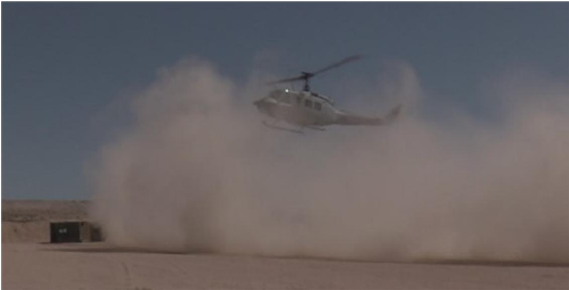
Figure 4.11: System Under Test Performing an Autonomous Landing During Full Brownout Conditions at Twentynine Palms Marine Base During Flight 59F120 [135]
