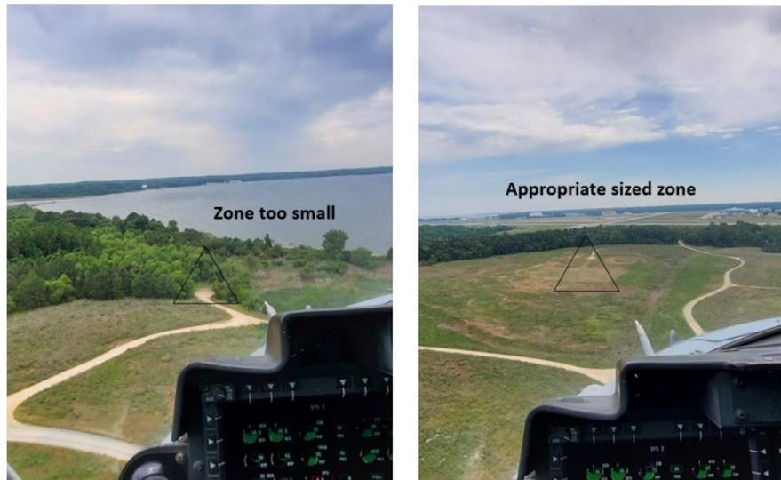
Figure 4.3: Pilots Perspective of Two LZs Taken From a UH-1 at 200 ft AGL Over the Turf Training Area of NAS Patuxent River [139]
