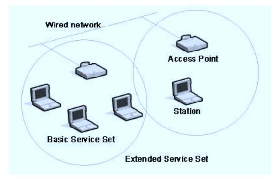
Figure 2: Architecture of the ESS mode.
