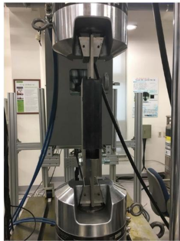
Figure 2.8 Experimental test setup of viscoelastic damper (Nasab and Kim [69])
