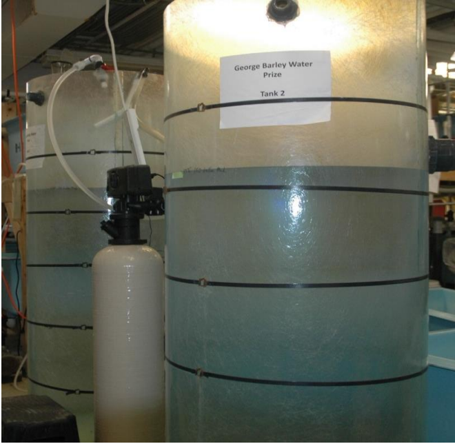
Figure 2.5 Image of the two-tank layout and fluidized sand filter filled with oolitic aragonite sand for the George Barley Water Prize trials.
