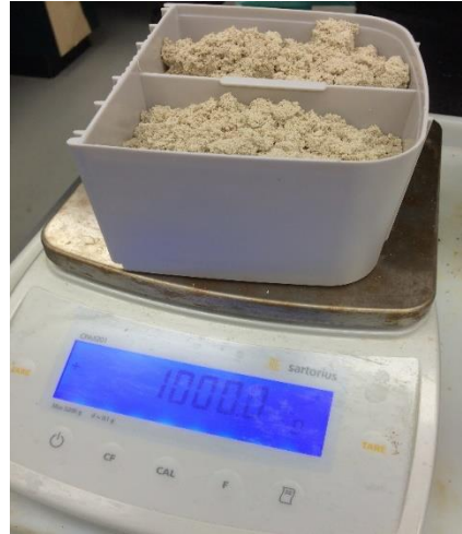
Figure 2.1 Internal compartment of Fluval® 406 canister filter holding 1000g of oolitic aragonite sand, as weighed on a scale.
