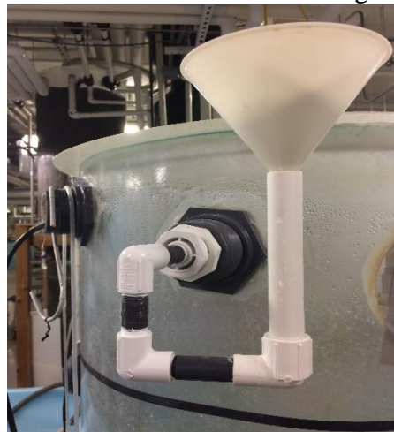
Figure 3.2 Additions port with funnel on side of reservoir tank. Piping filled with deionized water.
