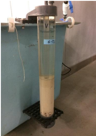
Figure 2.4 Image of the fluidized sand filter filled with gravel and 1000 g of oolitic aragonite sand and mounting position on end of fiberglass tank during a trial using brackish water.
