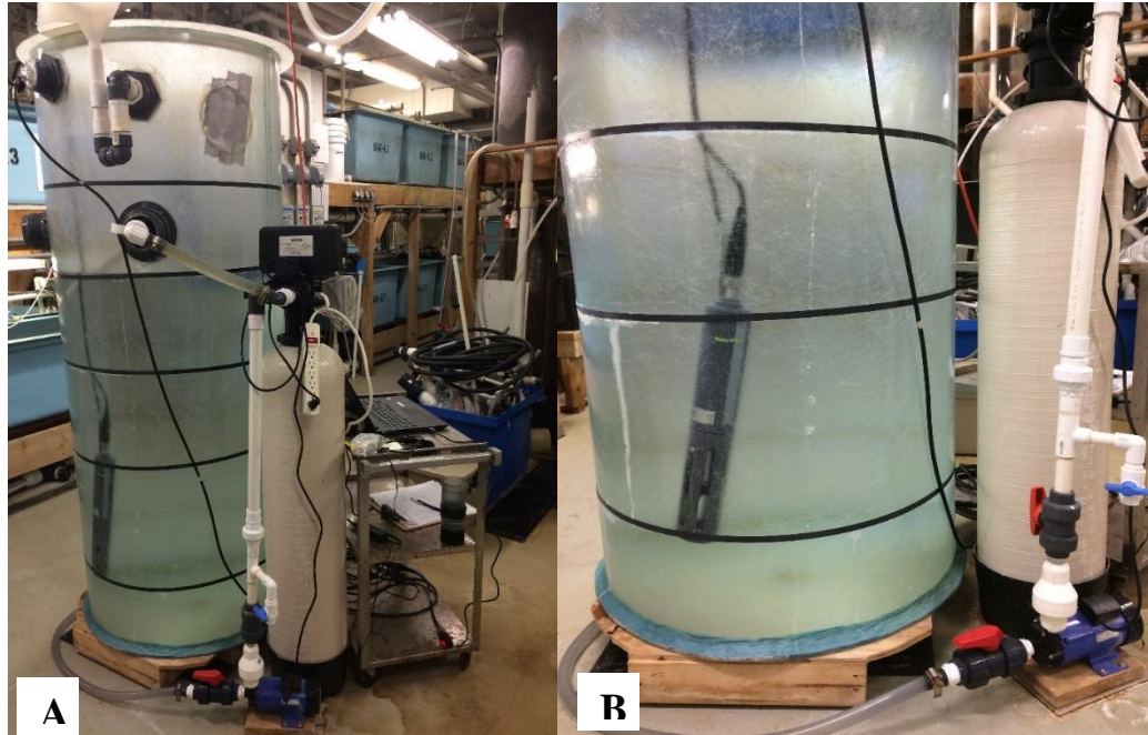
Figure 4.1 A. Arrangement of reservoir tank, circulation pump, fluidized sand filter, return to reservoir, addition port with funnel, monitoring probe in reservoir and computer recording data. B. Close-up of circulation pump, sampling port above pump and monitoring probe positioned in reservoir.
