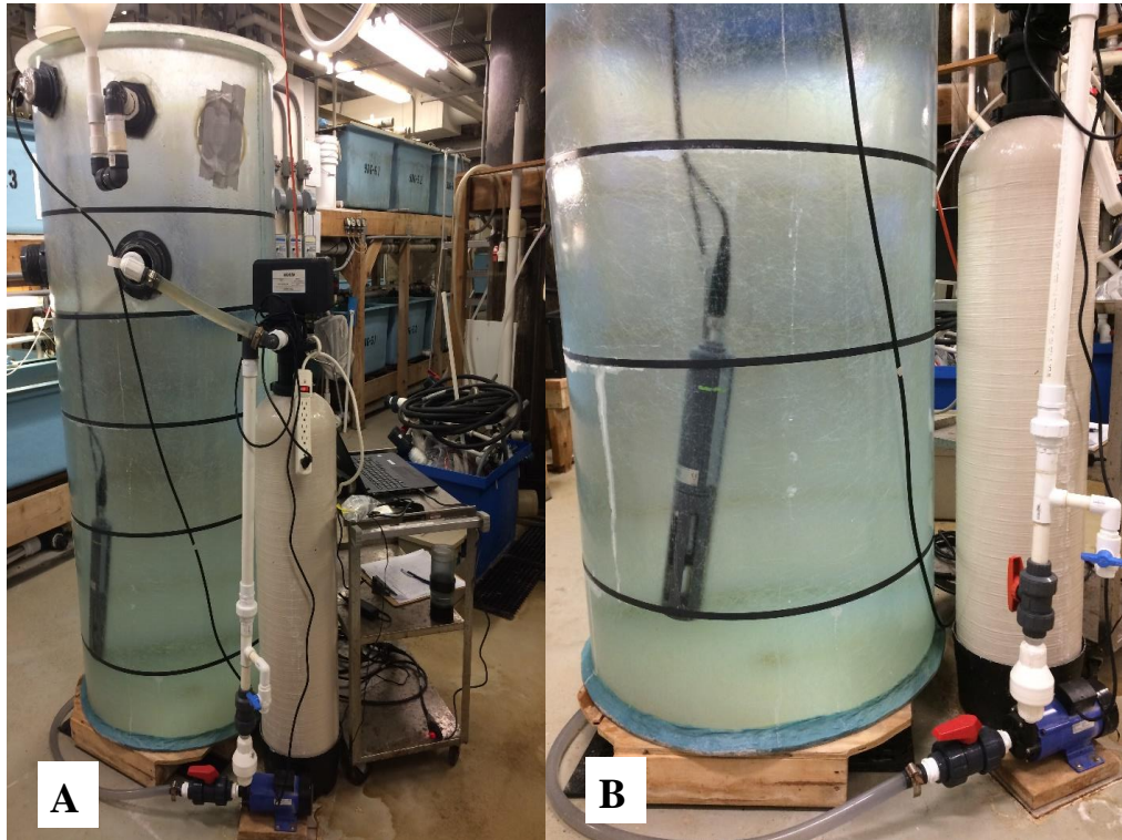
Figure 3.1 A. Arrangement of reservoir tank, circulation pump, fluidized sand filter, return to reservoir, addition port with funnel, monitoring probe in reservoir and computer recording data. B. Close-up of circulation pump, sampling port above pump and monitoring probe positioned in reservoir.
