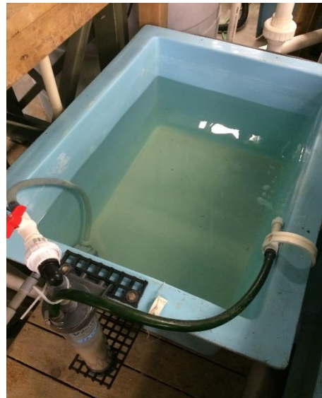
Figure 2.3 Image of fluidized sand filter placement, pump with control valve position and connection (left side) and filter return (right side) for a marine trial.
