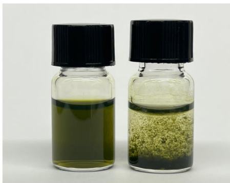
Figure 8.8 Probing NanoVP Electrostatic Stabilization. Representative digital images of NanoVP coated polymers. NanoVP was synthesized with (left) neutral polymer poloxamer 407 or (right) cationic polymer polyethylenimine. Poloxamer 407 had no impact on NanoVP stability, size, nor PDI. Polyethylenimine caused NanoVP to form large aggregates. N \geq 3 , where N equals the number of samples.
