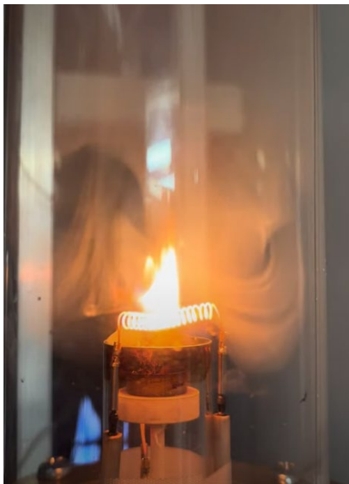
Figure 4.8 Smoke and air recirculation visible during MFC test on 200 mg of PVC with air co-flow of 7 SLPM.
