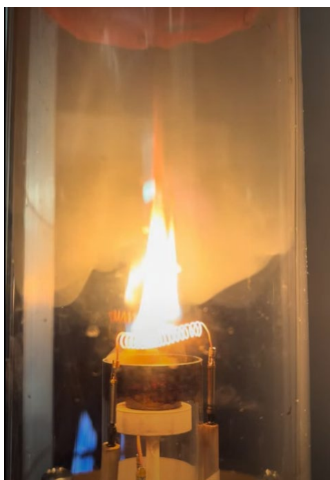
Figure 4.7 Smoke and air recirculation visible during MFC tests on 200 mg of PVC with air co-flow of 7 SLPM. Left: Quartz tube and exhaust hood in place without connection to sensors. Right: Open quartz tube, without exhaust tube or connection to sensors.
