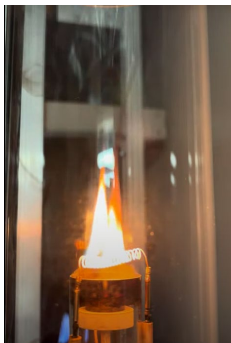
Figure 4.7 Smoke and air recirculation visible during MFC tests on 200 mg of PVC with air co-flow of 7 SLPM. Left: Quartz tube and exhaust hood in place without connection to sensors. Right: Open quartz tube, without exhaust tube or connection to sensors.
