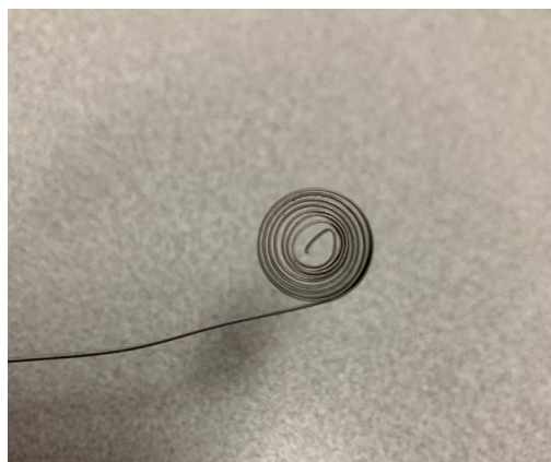
Figure 2.7 Coil made with Kanthal A1 3.17 mm x 0.32 mm wire using quilling tool.
