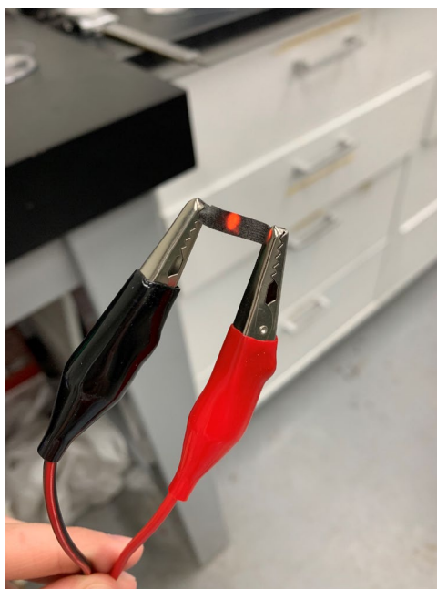
Figure 2.10 Strip carbon paper with a resistance of 6 \Omega pictured during testing at 6 V as it began to glow.
