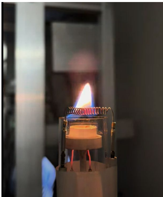
Figure 3.15 Open atmosphere test on 30 mg of PMMA powder with an N_2 flow rate of 250 sccm. Ignition was successful, but the flame location was unsteady, suggesting that samples at this small size experience some dilution from the N_2 flow.
