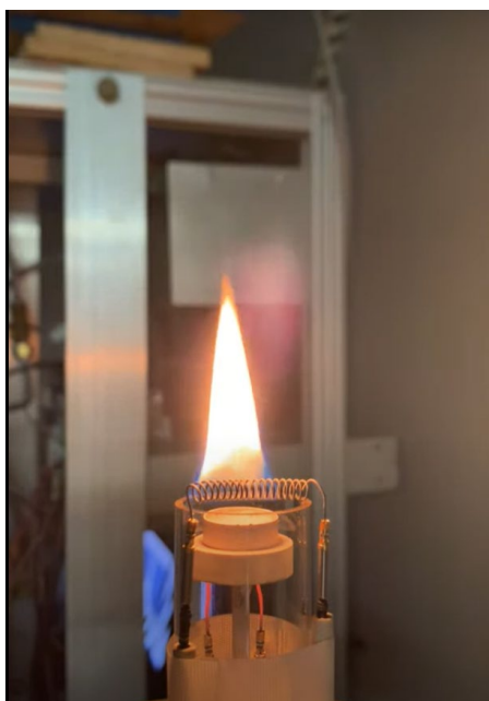
Figure 3.14 Open atmosphere test on 100 mg of PE with an N 2 flow rate of 250 sccm. The flame is located at the opening of the inner quartz tube and there is minimal visible condensation in the inner quartz tube.
