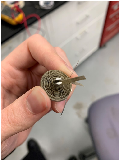
Figure 2.6 Kanthal A1 0.8 mm x 0.1 mm wire coiled using quilling tool.
