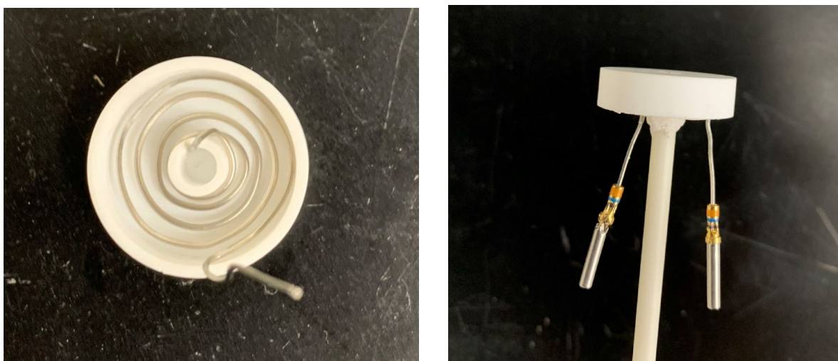
Figure 2.5 Left: Heating coil made of square 0.5 x 0.5 mm nickel chromium wire in ceramic heater. Right: Heater apparatus for updated MFC with attached thermocouple and wire leads.
