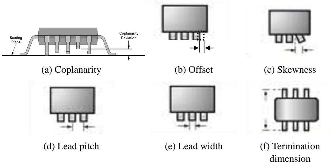
**Figure 7: Diagrams of definitions of measured conformity terms**
