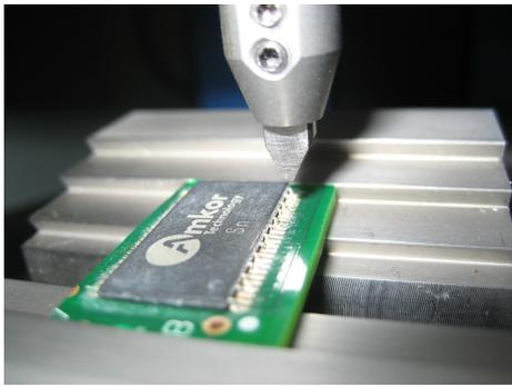
**Figure 26: Picture of shear test setup on DAGE 2400 Bondtester.**
