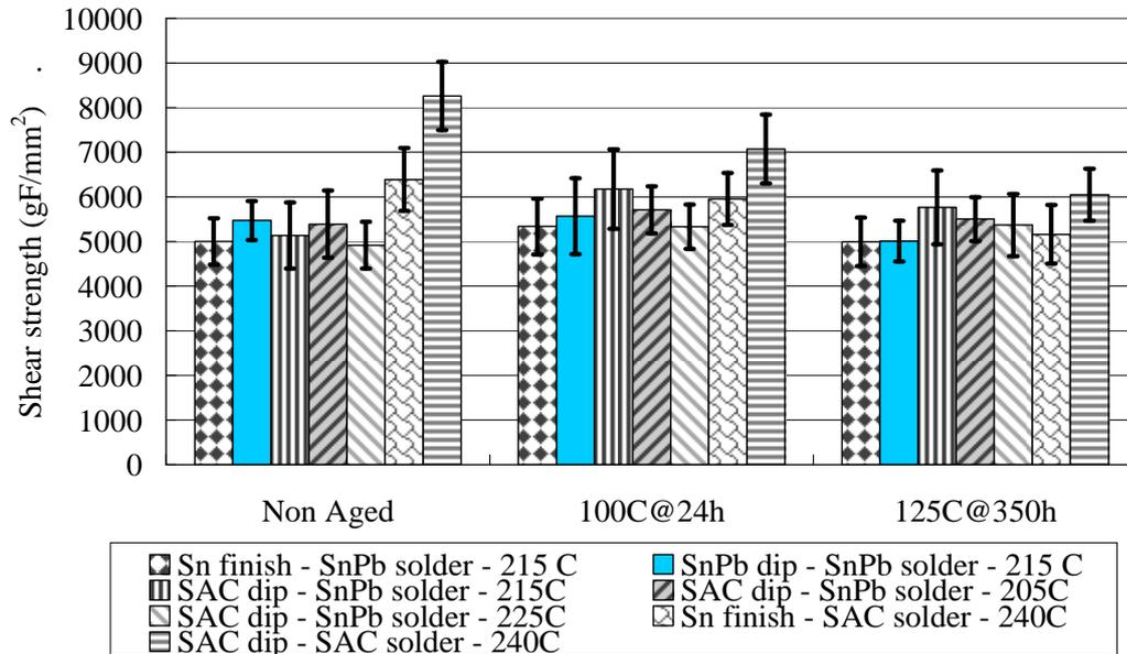
**Figure 28: Strength of solder joints reflowed with SnPb solder paste.**
