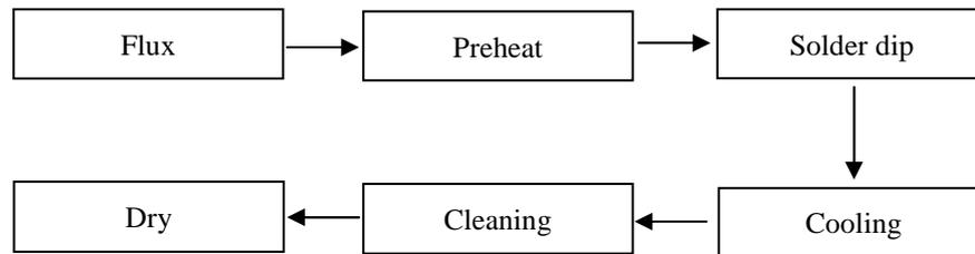
**Figure 1: Procedure of solder dip process**
