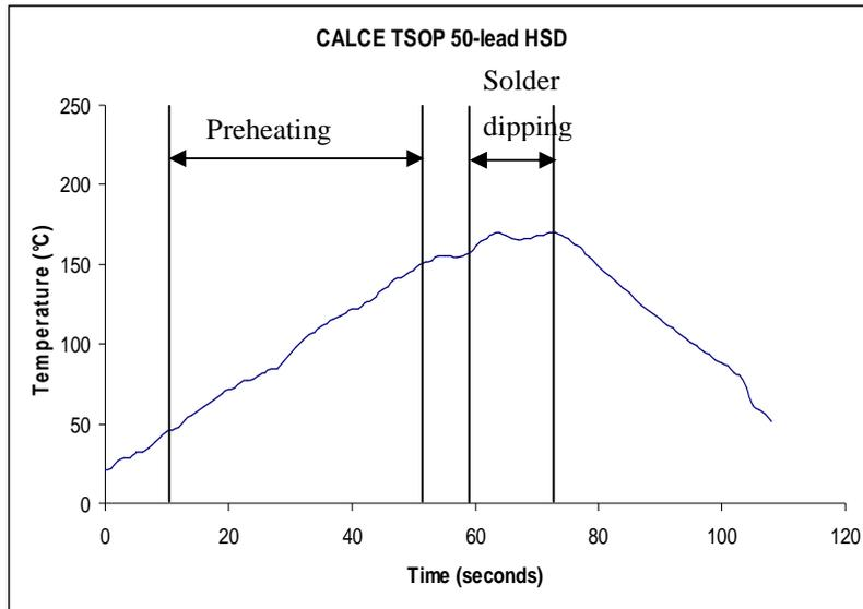
**Figure 4: Temperature profile of the SnPb solder dip process measured by a thermocouple**
