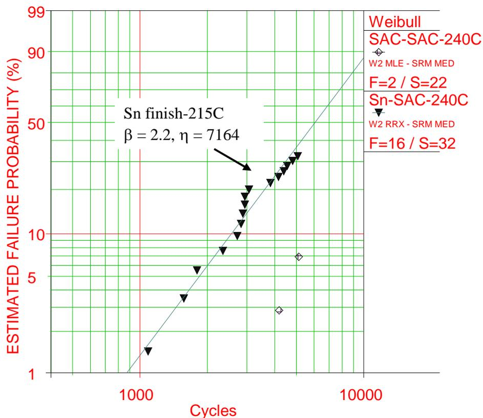
**Figure 34: Failure probability of solder joints of 2512 Resistor reflowed with SAC solder paste under temperature cycling test**
