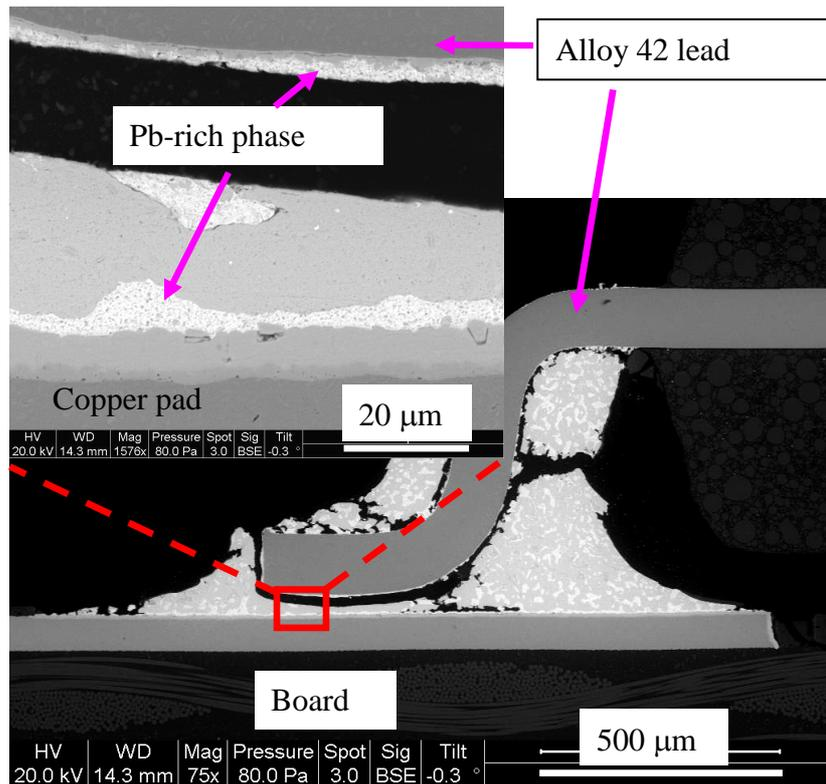
**Figure 40: Crack in TSOP solder joints: SnPb dip-SnPb solder-215°C-failed at 1366 cycles (corner solder joint)**
