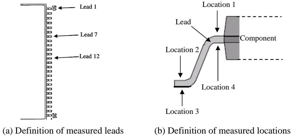
**Figure 9: XRF measurement sites on a TSOP component.**
