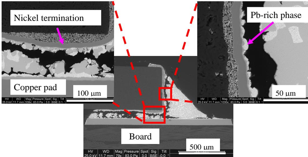
**Figure 41: Crack in resistor solder joints: SAC dip-SnPb solder-215°C-failed at 1655 cycles**
