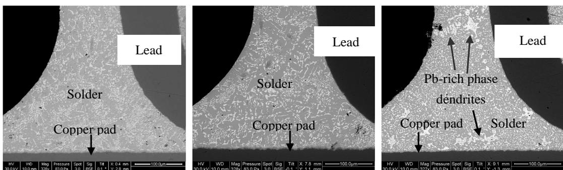
(a) Pure tin finished TSOP - SnPb paste – 215°C      (b) SAC dipped TSOP - SnPb paste – 215°C      (c) SnPb dipped TSOP - SnPb paste – 215°C
