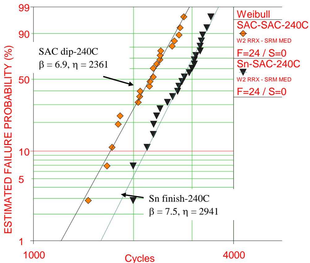
**Figure 33: Failure probability of TSOP solder joints reflowed with SAC solder paste under temperature cycling test**
