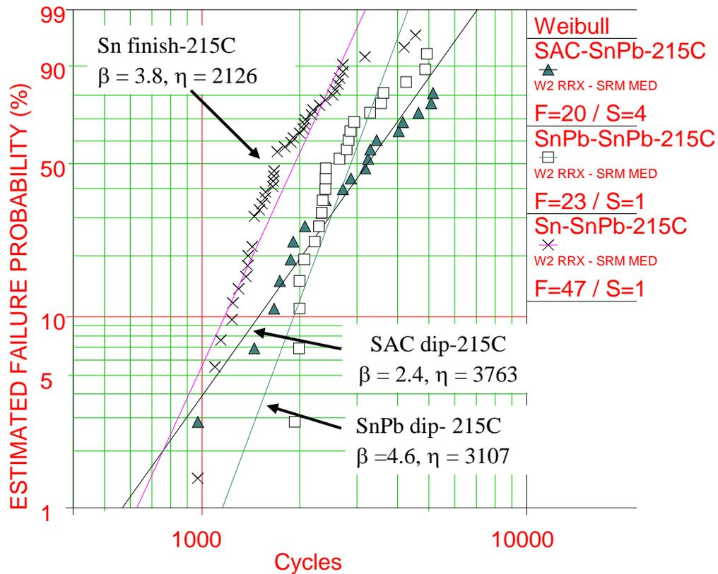
**Figure 32: Failure probability of 2512 Resistor solder joints reflowed with SnPb solder paste under temperature cycling test**
