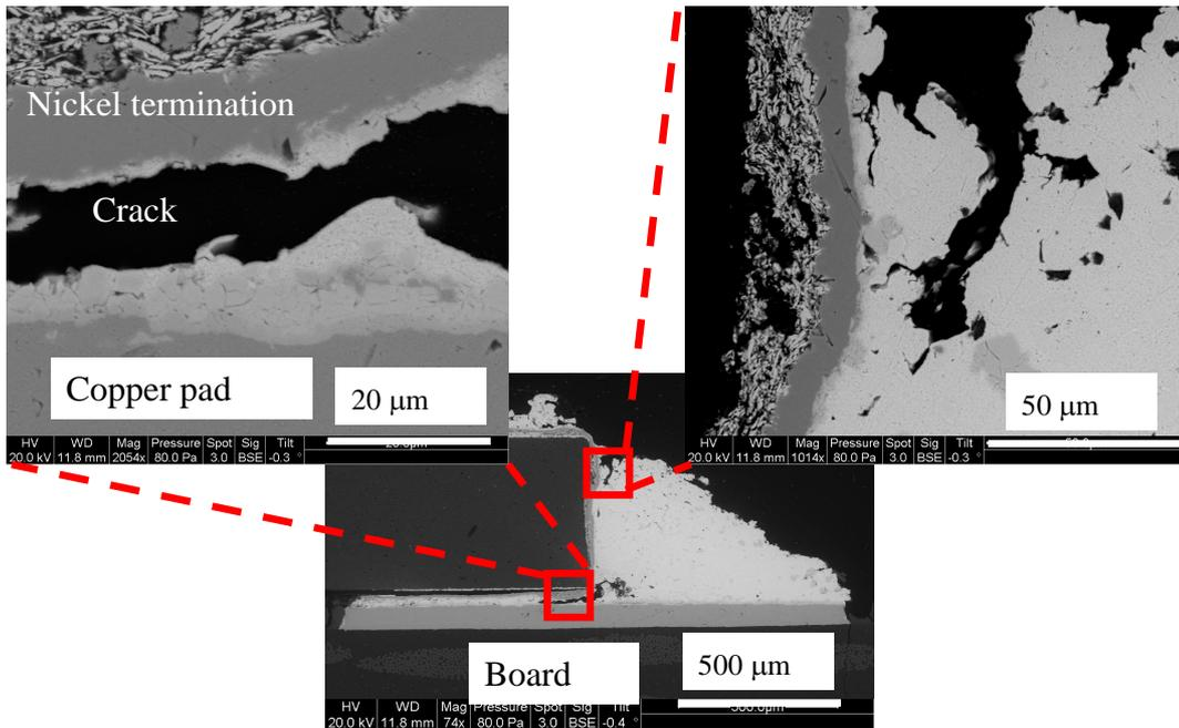
**Figure 44: Partial crack in resistor solder joint: SAC dip-SAC solder-240°C**
