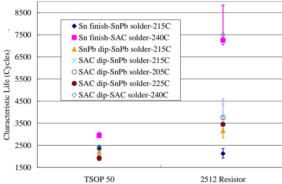
**Figure 45: Characteristic life of solder joints with 90% confidence intervals**
