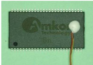
**Figure 3: A TSOP component attached with a thermocouple**
