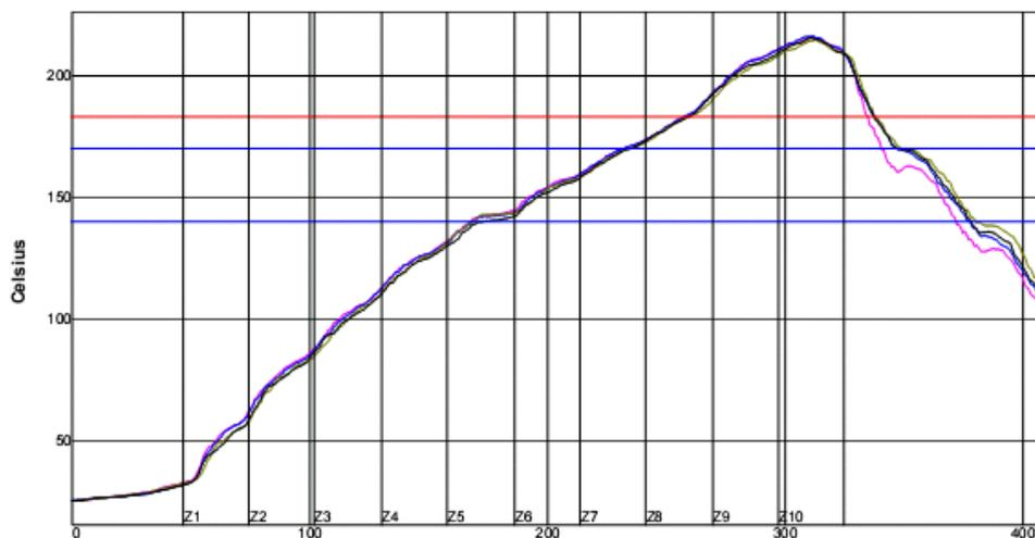
**Figure 11: Temperature profiles of reflow processes**
