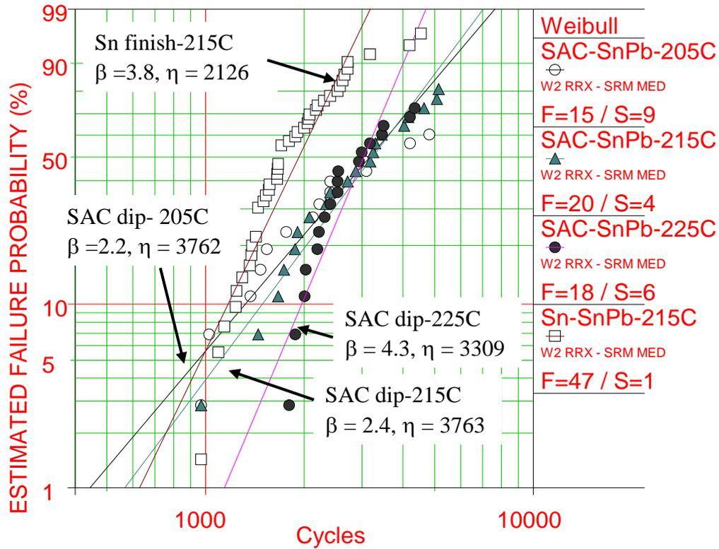
**Figure 36: Failure probability of solder joints formed with SAC dipped 2512 Resistor reflowed with eutectic SnPb paste under temperature cycling test**
