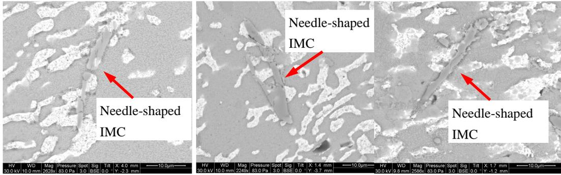
(a) Pure tin finished TSOP - SnPb paste – 215°C      (b) SAC dipped TSOP - SnPb paste – 215°C      (c) SnPb dipped TSOP - SnPb paste – 215°C
