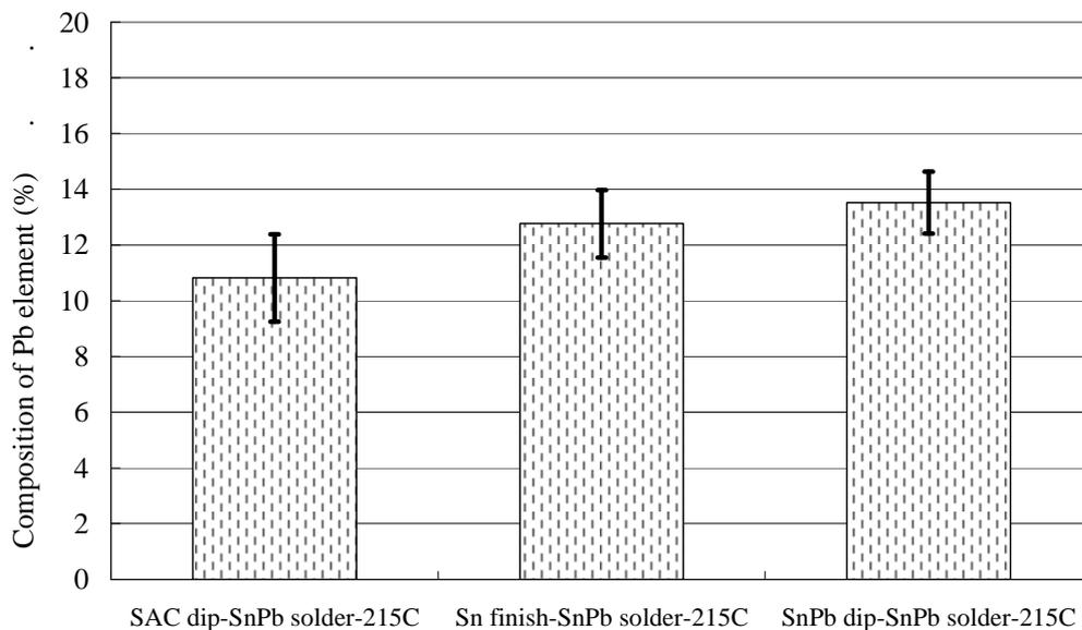
**Figure 17: Concentration of Pb element in TSOP solder joints assembled with SnPb solder paste.**
