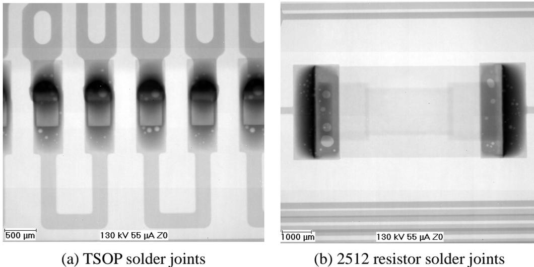
**Figure 13: X-ray pictures of TSOP solder joints and resistor solder joints: SAC dip – SAC solder – 240C**
