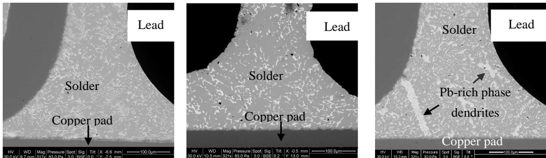
(a) Pure tin finished TSOP - SnPb paste – 215°C      (b) SAC dipped TSOP - SnPb paste – 215°C      (c) SnPb dipped TSOP - SnPb paste – 215°C
