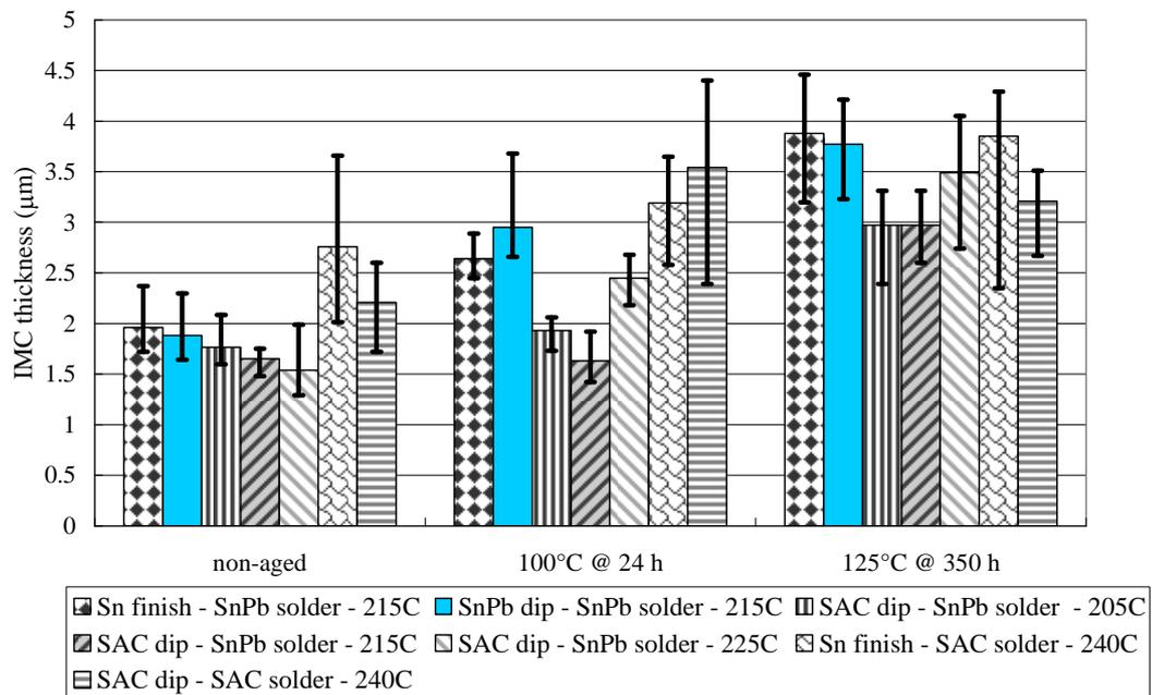
**Figure 23: IMC layer thickness at the interface between the solder and the board copper pad in solder joints formed with Sn finished, SAC dipped and SnPb dipped TSOPs.**
