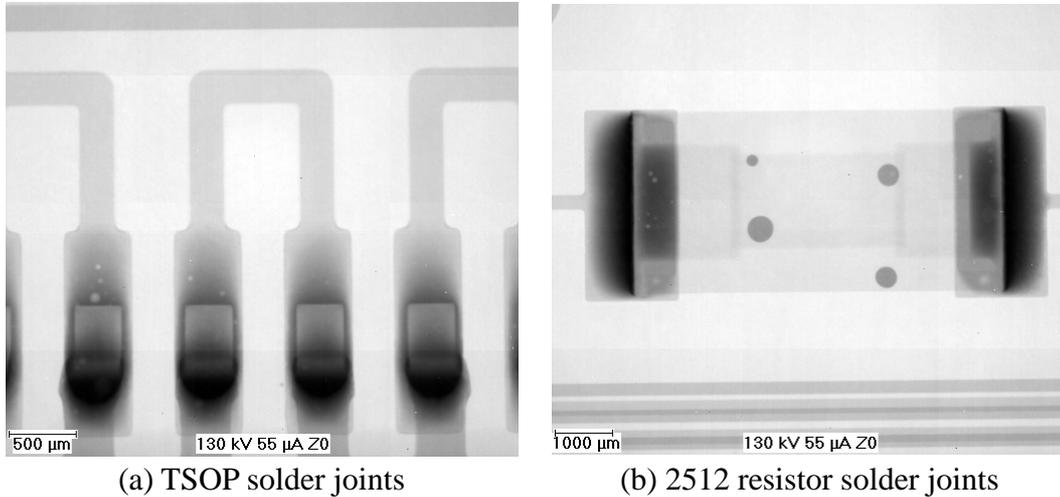
**Figure 12: X-ray pictures of TSOP solder joints and resistor solder joints: SAC dip – SnPb solder – 215C**
