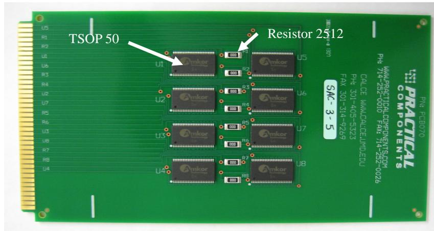
**Figure 10: Optical picture of test board**
