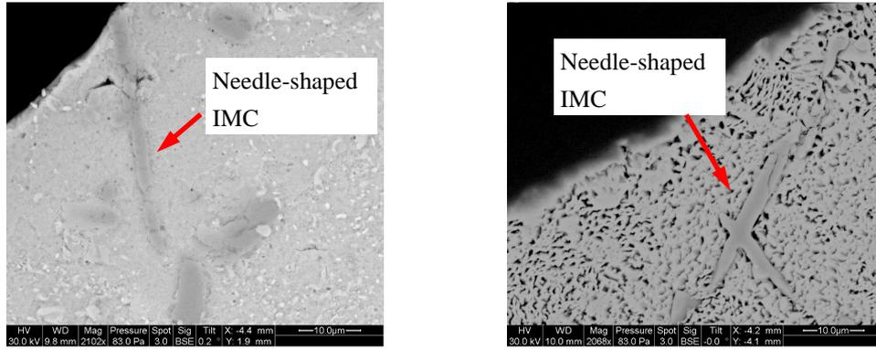
(a) Pure tin finished TSOP - SAC paste – 240°C      (b) SAC dipped TSOP - SAC paste – 240°C
