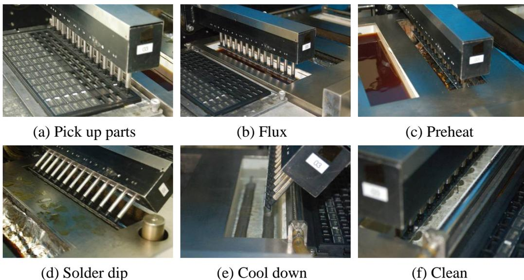
**Figure 2: Pictures of solder dip process**
