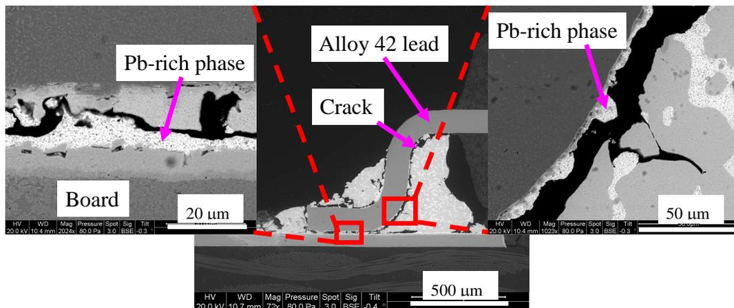
**Figure 39: Crack in TSOP solder joints: SAC dip-SnPb solder-215°C-failed at 1136 cycles (non-corner solder joint)**
