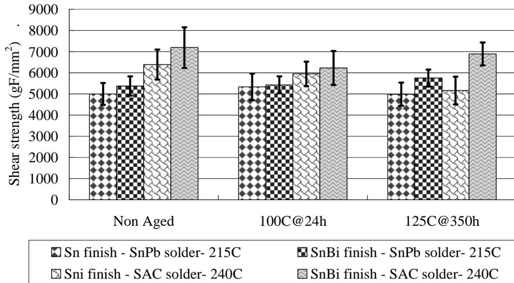
**Figure 29: Shear strength of solder joints formed with SnBi finished TSOPs and pure tin finished TSOPs.**
