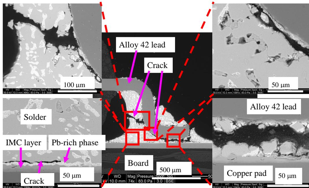
**Figure 38: Crack in TSOP solder joints: SAC dip-SnPb solder-215°C-failed at 2216 cycles (corner solder joint)**
