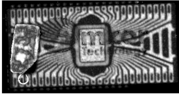
**Figure 6: C-SAM image of the interface between die surface and molding compound with 75Hz transducer**
