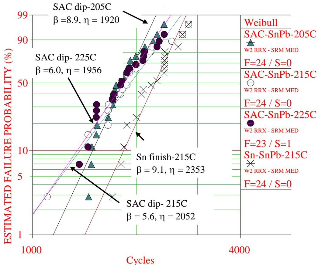
**Figure 35: Failure probability of TSOP solder joints formed with SAC dipped TSOPs reflowed with SnPb solder paste under temperature cycling test**
