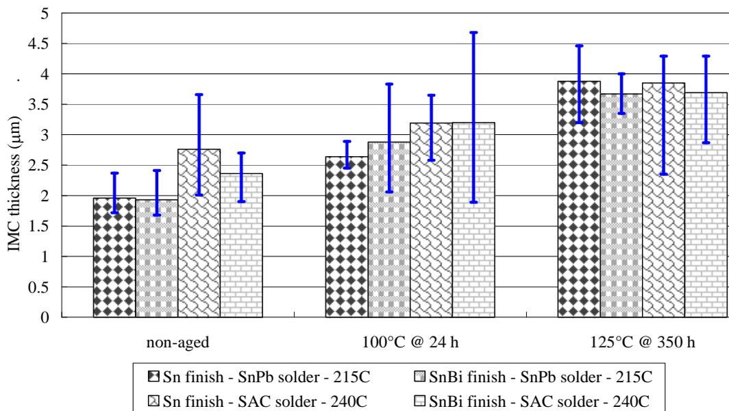
**Figure 24: IMC layer thickness at the interface between the solder and the board copper pad in solder joints formed with Sn finished and SnBi finished TSOPs.**
