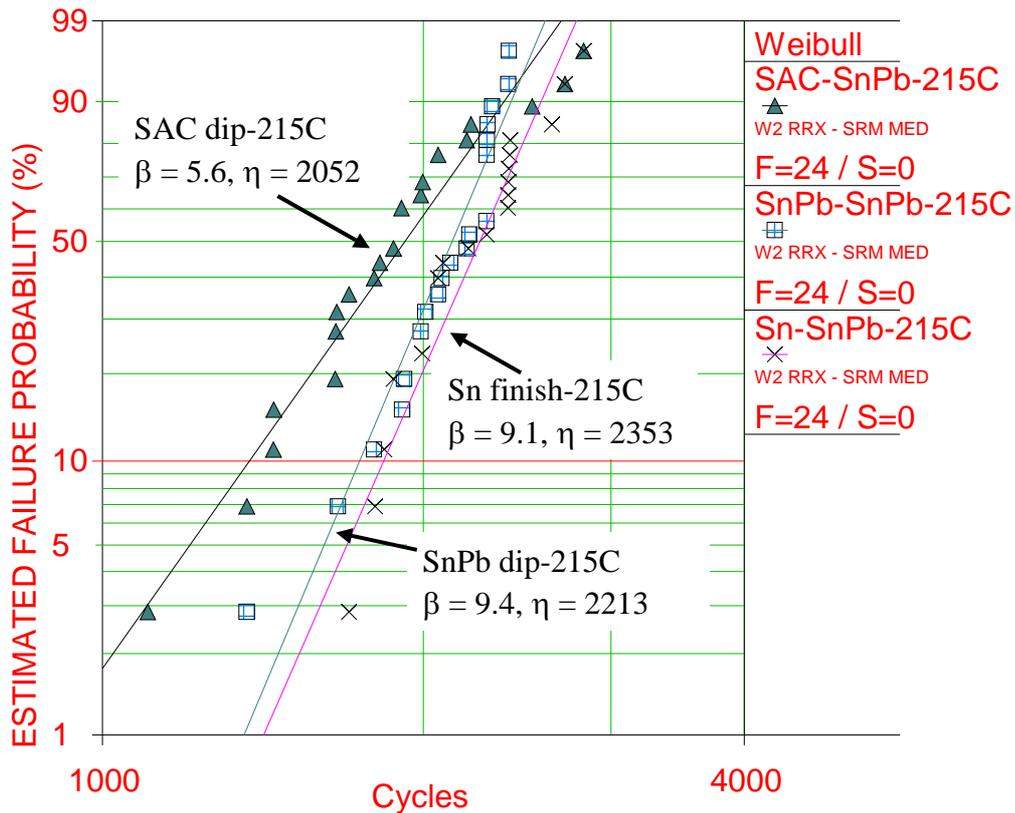
**Figure 31: Failure probability of TSOP solder joints reflowed with SnPb solder paste under temperature cycling test**
