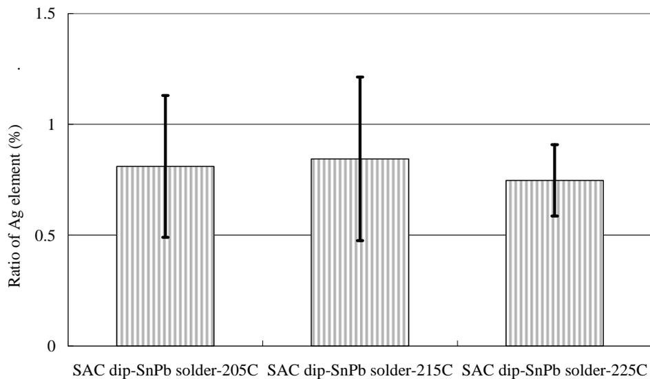
**Figure 25: The ratio of Ag element in the solder joints formed with SAC dipped TSOPs assembled with SnPb solder paste (Non-aged)**
