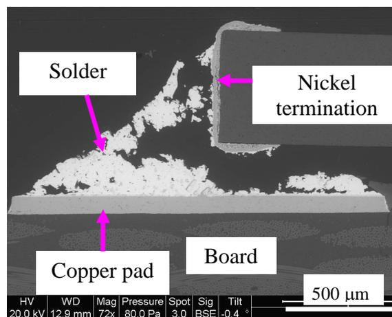
**Figure 43: Cracks in resistor solder joints: SAC dip-SAC solder-240°C-4182 cycles**
