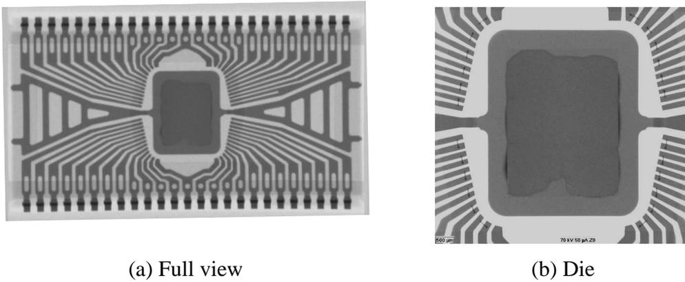
**Figure 5: X-ray images of TSOP component before solder dip**
