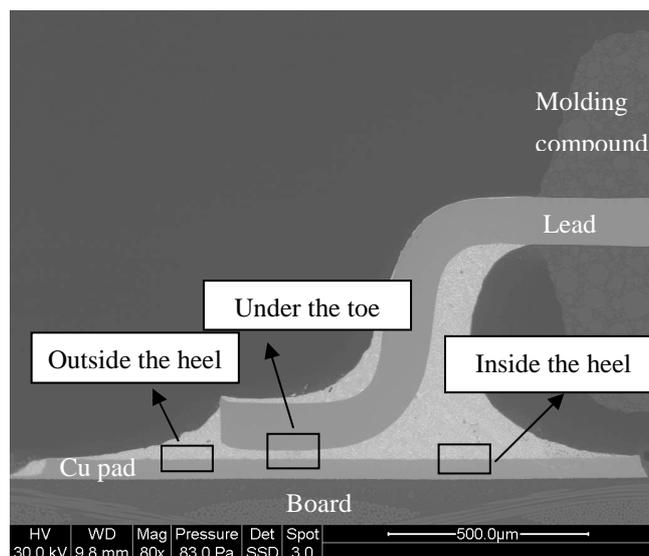
**Figure 22: Locations investigated for IMC thickness in a solder joint.**
