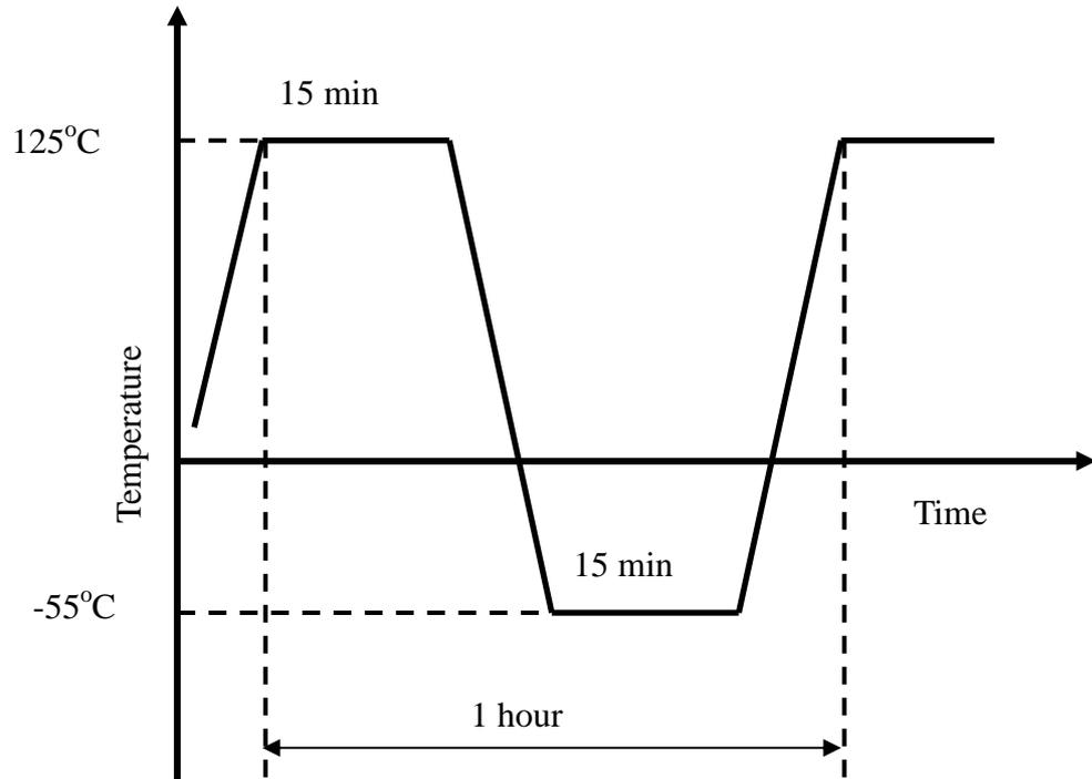
**Figure 30: Temperature profile of temperature cycling test**
