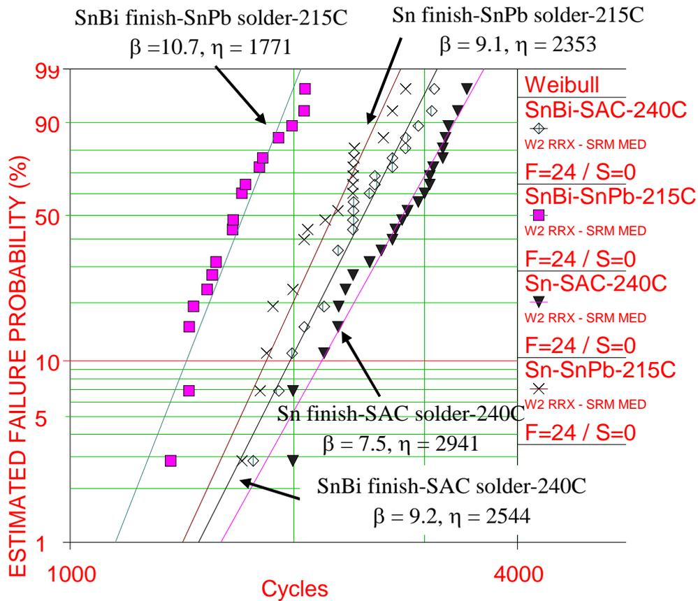
**Figure 37: Failure probability of solder joints formed with original pure tin finished and original SnBi finished TSOPs under temperature cycling test**
