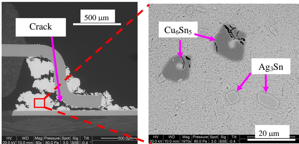
**Figure 42: Cracks in TSOP solder joints: SAC dip-SAC solder-240°C-1461 cycles**
