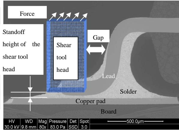
**Figure 27: Diagram of shear test setup.**
